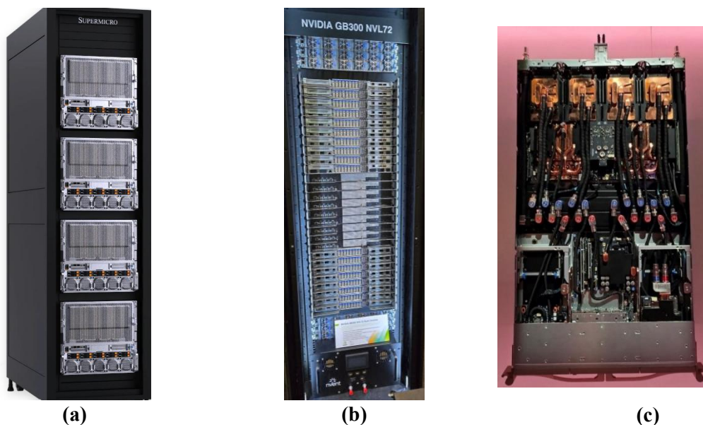
Figure 1: Reference architectures: (a) Air-cooled design: Supermicro HGX B200 rack with four 10U compute server. (b) Liquid cooled design: NVIDIA GB300 rack layout with (c) 1U compute server tray.
