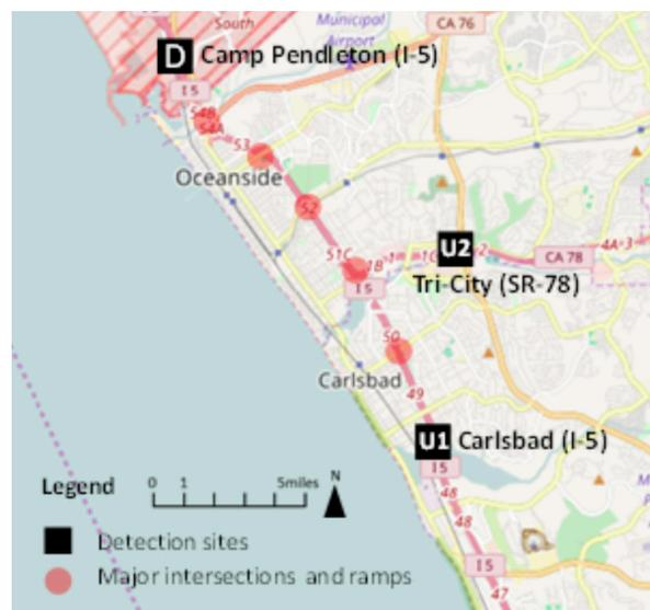
Figure 2. Truck signature data was collected at two upstream locations (U1 and U2) and one downstream location (D) in Southern California. TAMS observed 284 trucks (i.e., matched the truck signatures) that passed through either one of the upstream locations and the downstream location.
