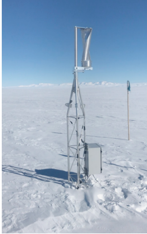
Figure 2.26: Photo of the vertical axis wind turbine, developed at Uppsala University, which was deployed during the Antarctic summer of 2017-2018, and has provided power to ARI-ANNA site E throughout the winter.
