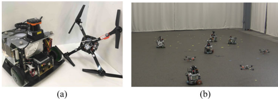
Fig. 3. (a) A Scarab ground robot and a Hummingbird quadrotor. (b) The experimental setup with 3 UAVs and 5 Scarabs.
