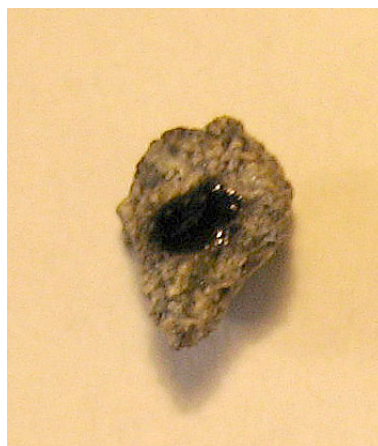
Figure 5.8: Image of lunar specimen 62235.119 after exposure to microwave energy equivalent to 144 watt-secs. The dark circle in the center of the specimen is a glassy and most likely a melt bubble produced during decay of spin waves generating heat through lattice vibrations within the bulk specimen.
