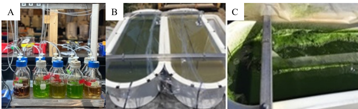
Figure 13. Microalgae cultivation at different scales: (A) 300mL lab scale cultivation; (B) 100L open pond algae cultivation reactors at UC Davis, covered with clear 0.7-mm-thick plastic; (C) high density algae culture grown in 10% filtered food waste digestate.
