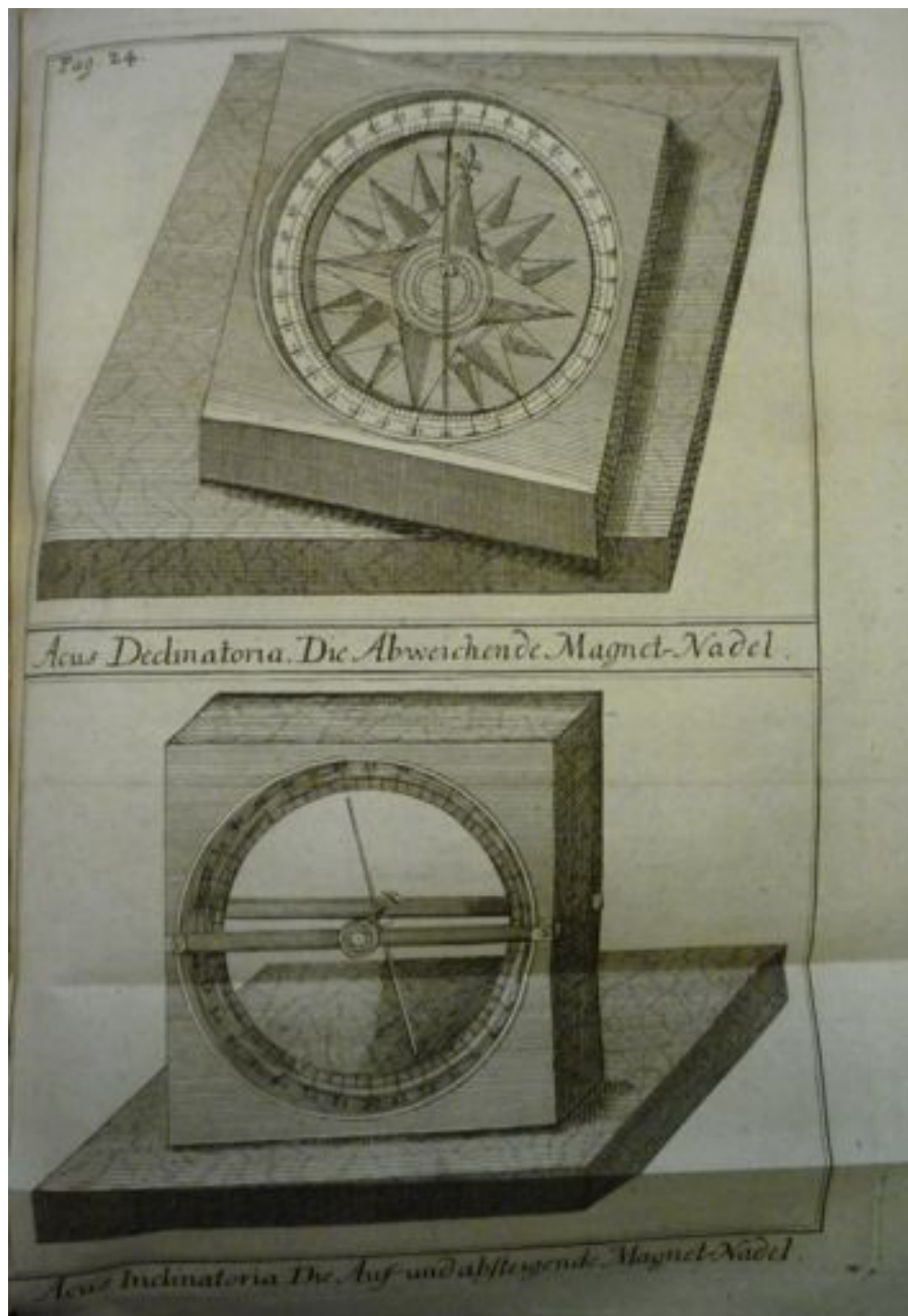
Figure 7: Eberhard's engravings of a regular and an inclinatory compass.
