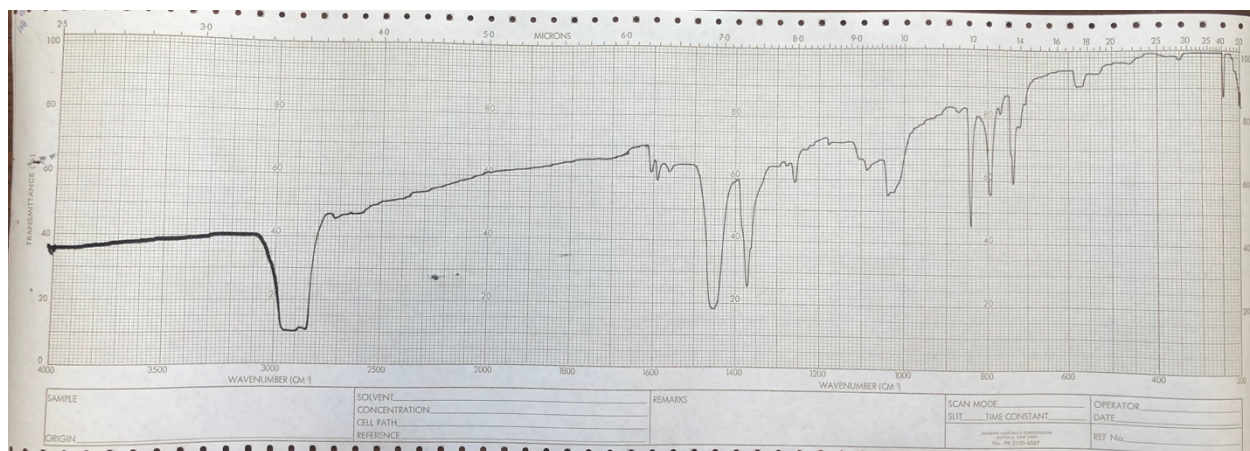
Figure S3.3 Infrared spectrum of a Nujol mull of \{\text{Cu}_2(\text{SAr}^{\text{Me6}})\text{Mes}\}_2 ( 1 ) at 25°C
