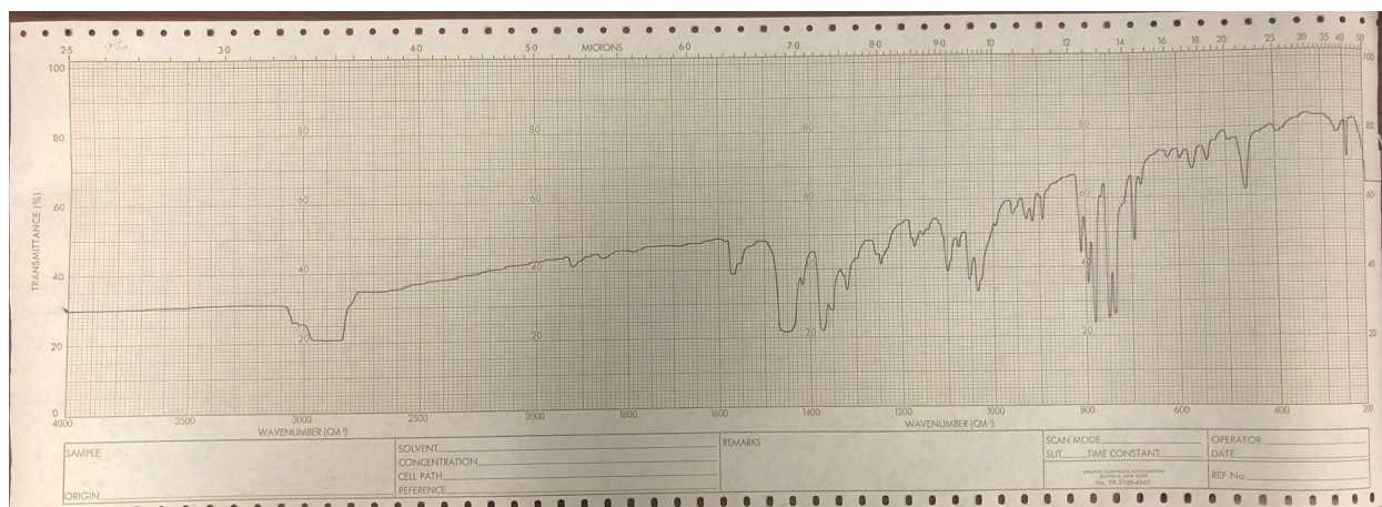
Figure S2.3 Infrared spectrum as a Nujol mull of \{\text{CuSAr}^{\text{iPr}_4}\}_2 ( 1 ) at 25°C
