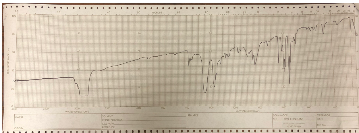
Figure S3.7 Infrared spectrum of a Nujol mull of \{\text{Cu}_2(\text{SAr}^{\text{iPr}_4})\text{Mes}\}_2 ( 2 ) at 25°C
