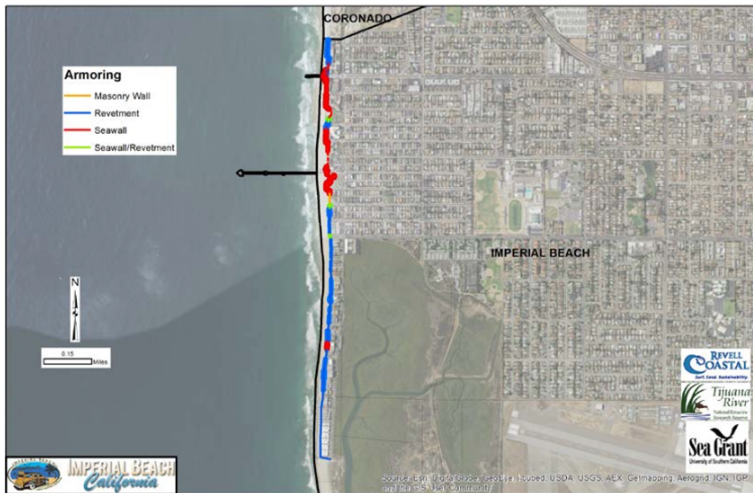
Figure 2. Coastal armoring in IB, classified by type (Revell Coastal 2016)
