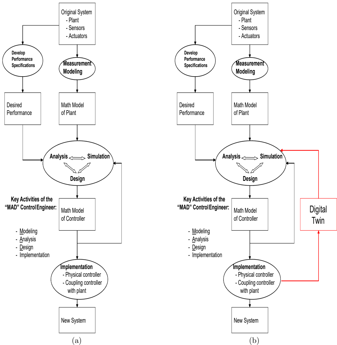
Figure 6.1: Modeling, Analysis, and Design (MAD) Methodology for Control Engineering (a) Classic Approach and (b) MAD Enabled with Digital Twin
