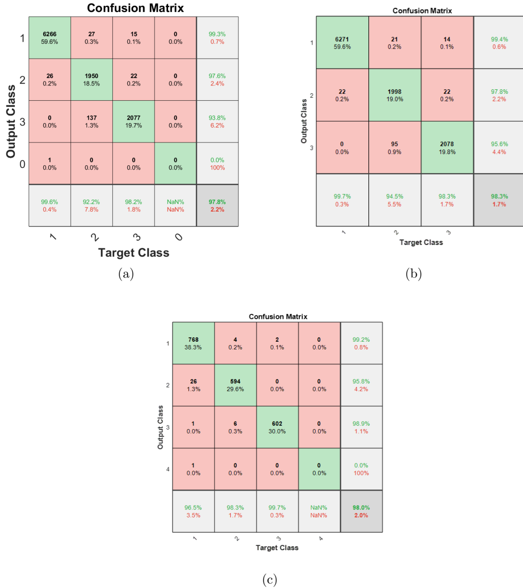
Figure 6.13: Artificial Neural Network Fault Detector Confusion Matrices a) Training b) Validation (Synthetic Data) c) Cross Validation (Real Fault Dataset)
