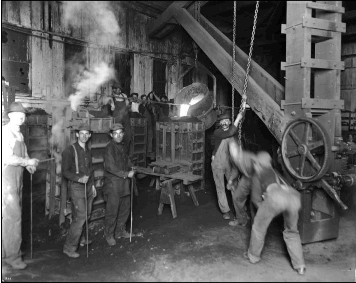
Figure 5.14. Skilled labor casting molten iron at Judson Manufacturing Company (or bolt works?). Source: Emeryville Historical Society.
