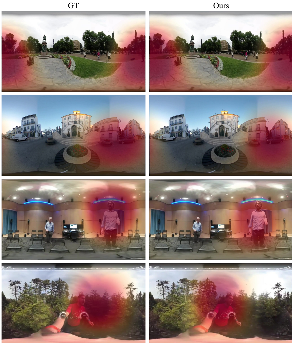
Figure 5.4: Qualitative Results. Comparison between predicted and recorded FOA. Spatial audio is visualized as a color overlay over the frame, with darker red indicating locations with higher audio energy.
