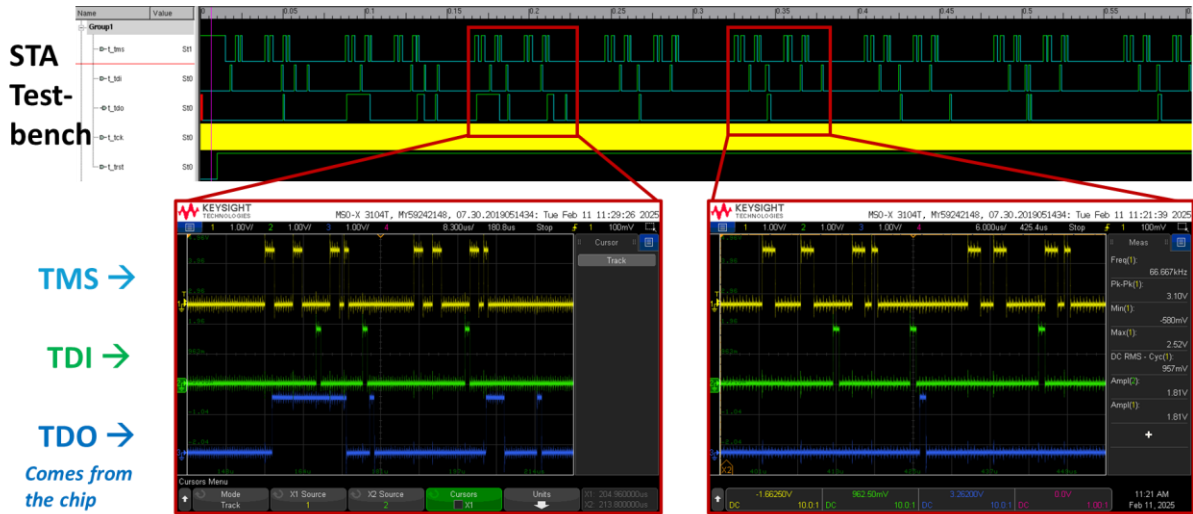
Figure 5.25 Comparison of STA waveforms with the actual waveforms obtained from the Anuvāda chip showing a perfect match. These inputs (TDI/TMS) and outputs (TDO, obtained from chip) are used to configure the PCIe block.
