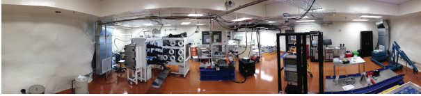
FIGURE 11: A view of the detector laboratory at the Davis Campus at SURF. In this view, the glove box is to the left, and the prototype module is at the center. In the rear, a soft-wall cleanroom is shown that serves the purpose of an area of increased cleanliness.
