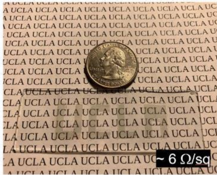
Figure 5-3. Optical image of printed AgNW pattern on glass (sheet resistance: 6 Ohm/sq )
