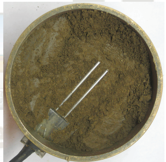
Fig. 1. The rigid dual-probe heat-pulse (R-DPHP) sensor, with probes that are 2.38 mm in diameter and 40 mm in length (R-DPHP-40), after excavation of the Yolo silt loam at a volumetric water content of 0.23 \text{ m}^3 \text{ m}^{-3} .
