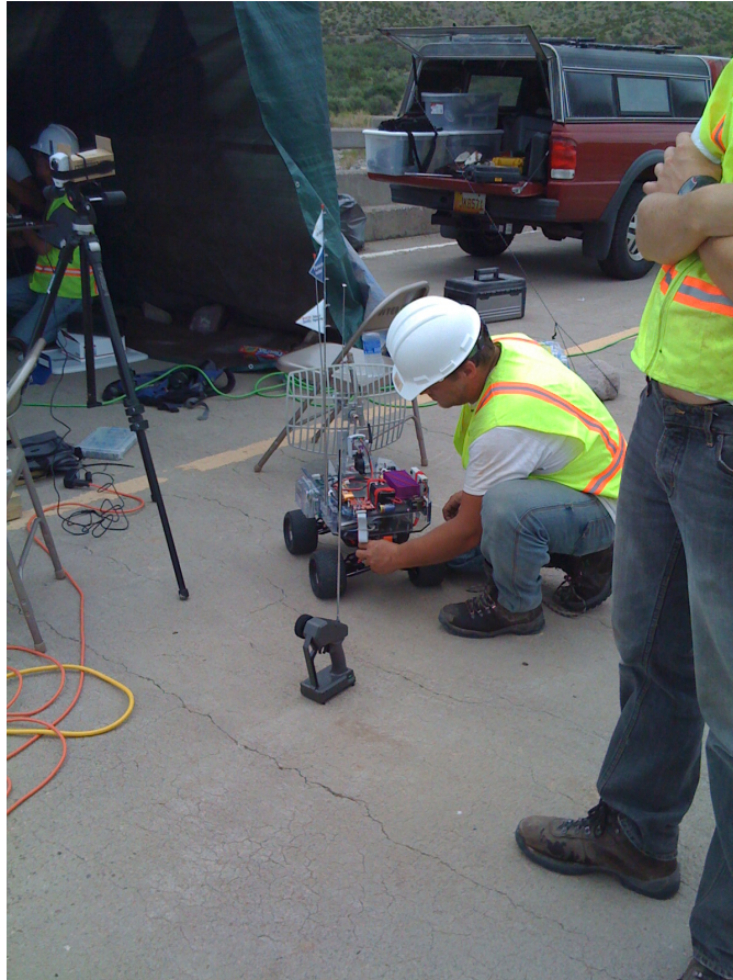
Figure 3.5: Remote Controlled Robot Used for Collecting SHM Data
