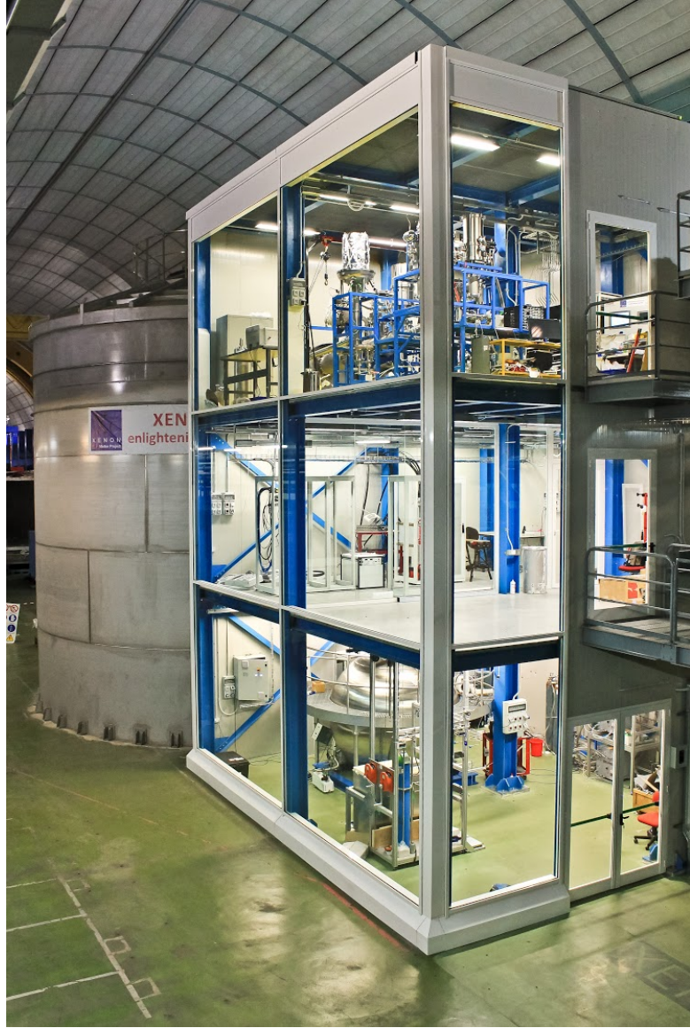
Figure 2.2: XENON1T water tank and associated facilities. The cryogenic and circulation system and connection to the TPC through water tank is on the third floor; all the electronics such as data acquisition system will be on the second floor; xenon storage is on the ground floor. This picture is taken by P. DePerio from Columbia University.
