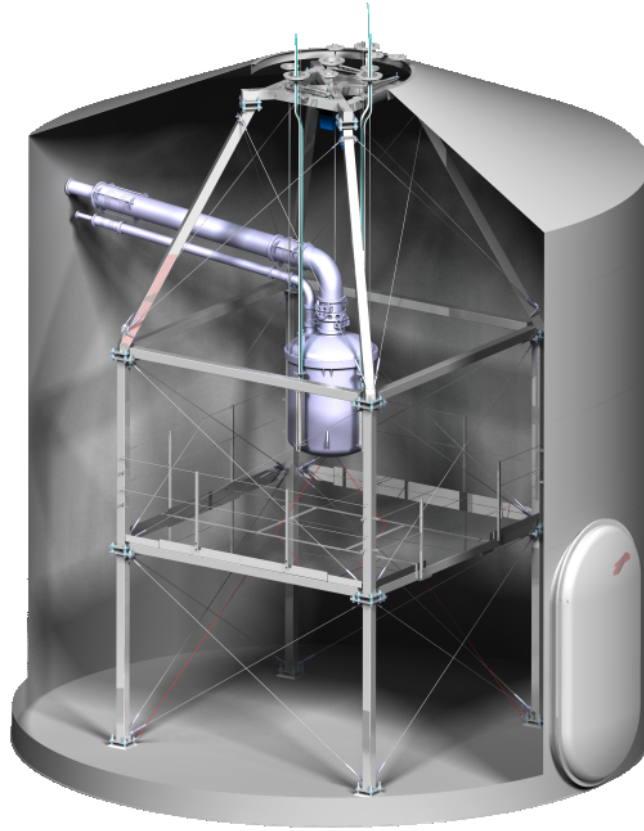
Figure 2.3: A 3D drawing of XENON1T TPC inside the water tank. The connection to the TPC through a port is from the adjacent service building, which is shown in the Figure 2.2.
