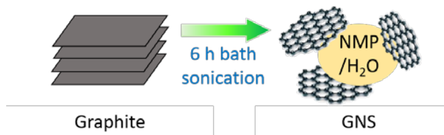
Figure 2.5 Schematics of GNS exfoliated from bulk graphite using an 8:2 NMP/H 2 O solvent.
