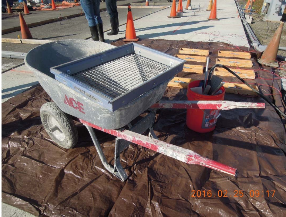
Figure A.79: Sieve for preparing the unrestrained shrinkage beams.
