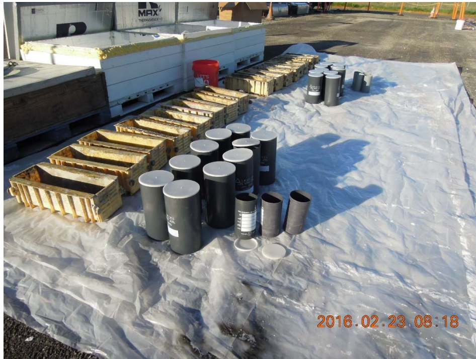
Figure A.45: Cylinder and beam molds for QC/QA specimen preparation.
