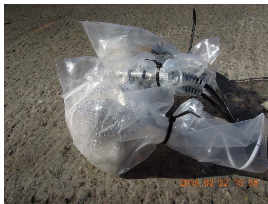
Moisture conditioning of RH and moisture content sensors
