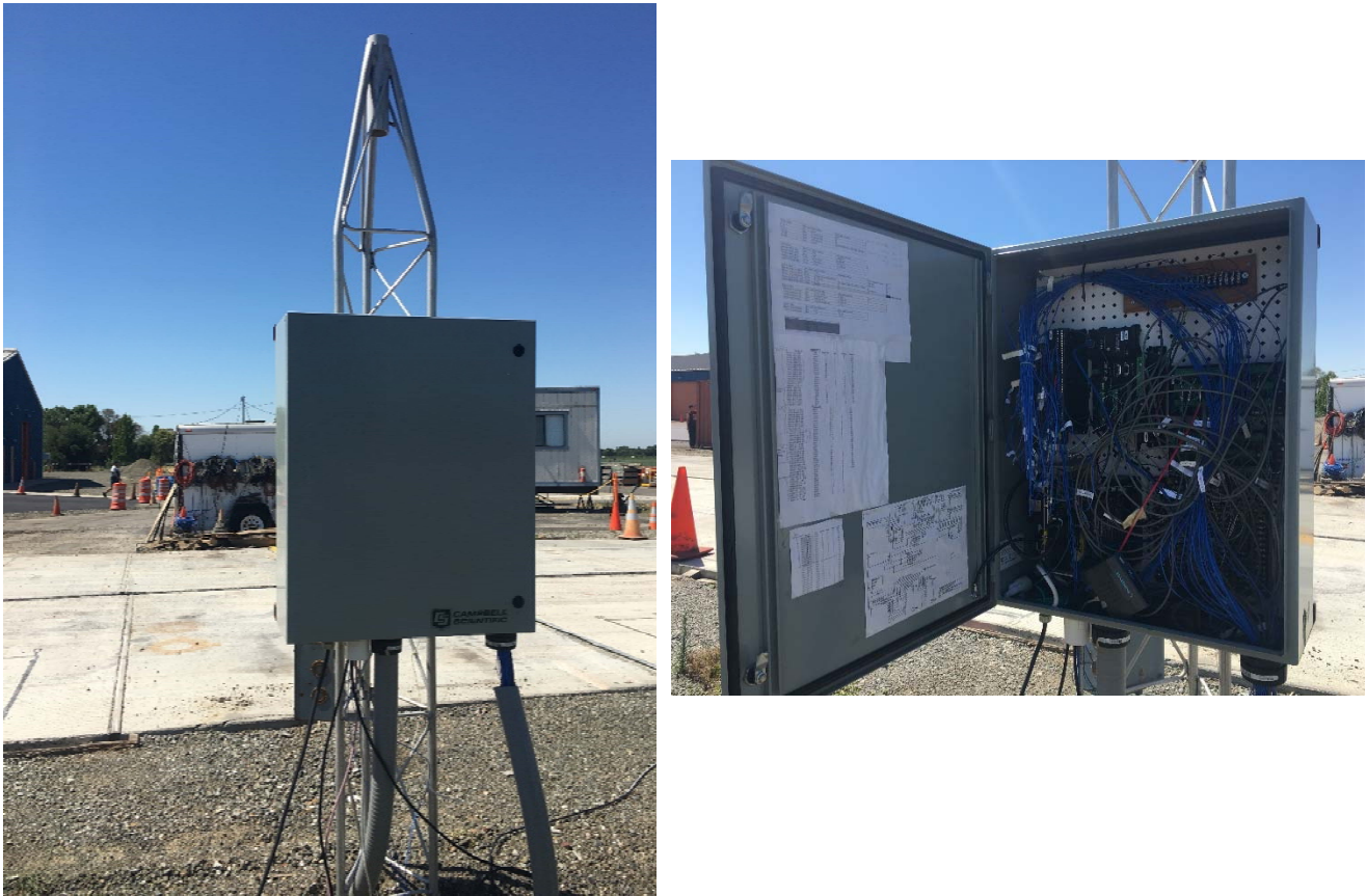
Figure 3.16: Pictures of one of the Campbell Scientific data acquisition systems.
