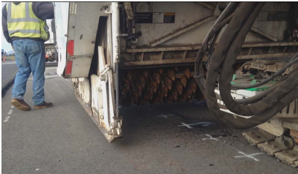
Figure A.9: Milling machine with micromilling teeth spacing.
