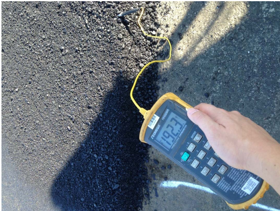
Figure A.6: Temperature tracking inside the HMA.
