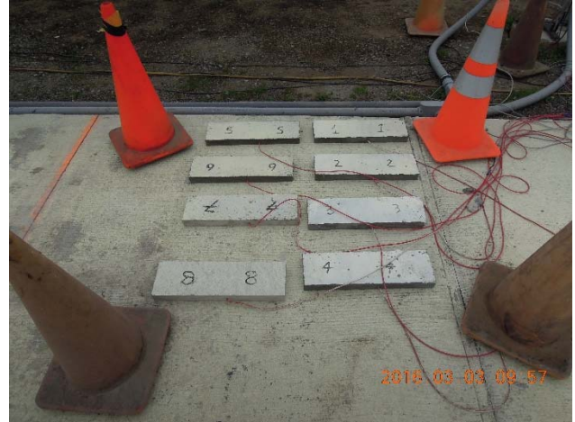
Beams after demolding
