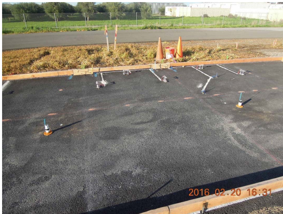
Figure A.14: Layout of instruments in an HVS section.
