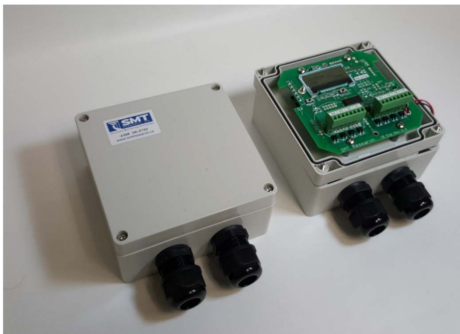
Figure 3.17: Photos of the A3 NEMA data logger from SMT Research.
