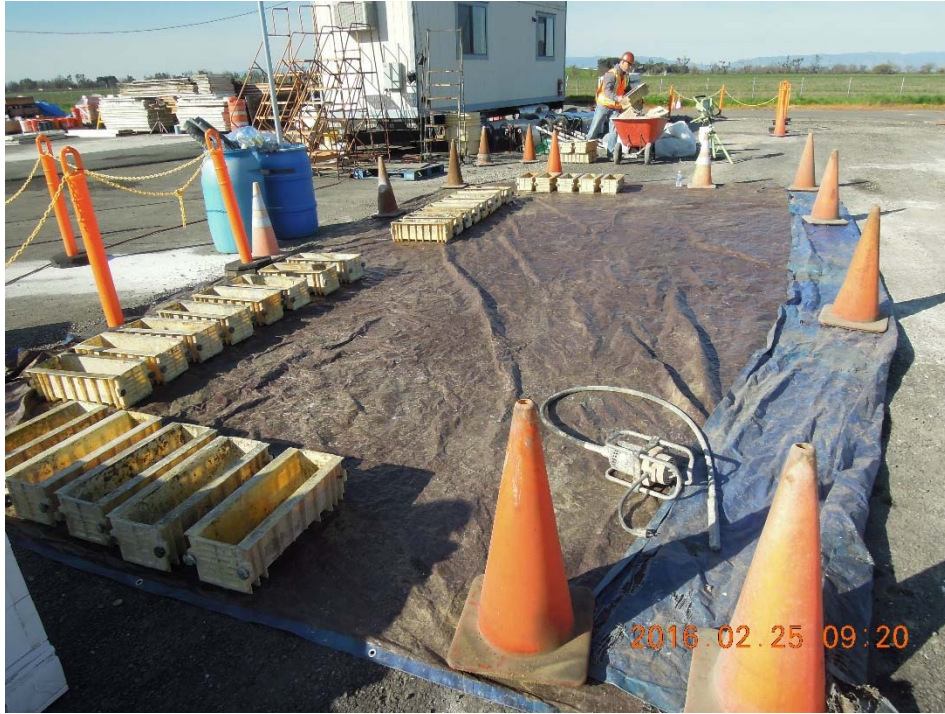
Figure A.81: Flexural beam molds.
