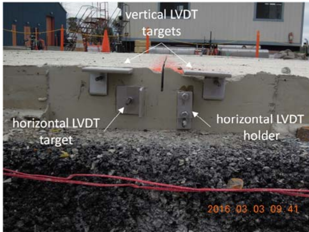
Figure 3.13: JDMD targets and horizontal JDMD holder.
