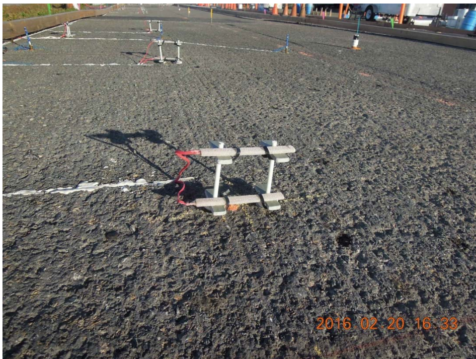
Figure A.16: Close-up of dynamic strain gages.
