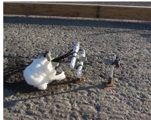
From left to right: two moisture content sensors (the bottom one is under the wet paper towel), two RHC sensors, and one RHS sensor
