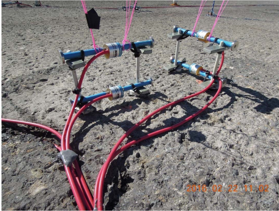
Figure A.21: Close-up of longitudinal and transverse static strain gages.
