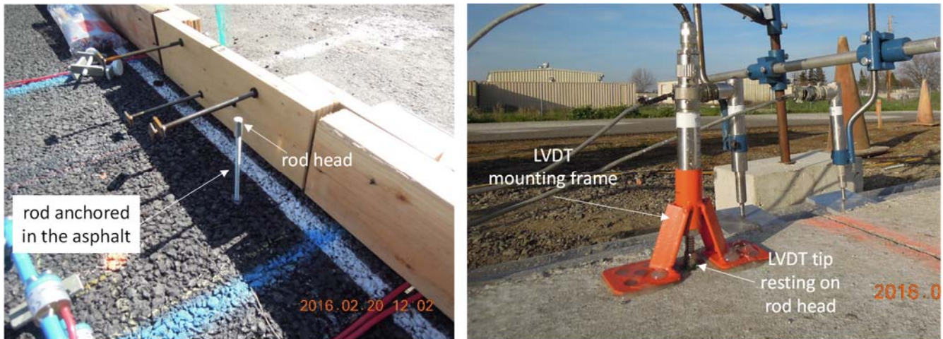
Figure 3.14: Interface opening measuring device (IOMD).
