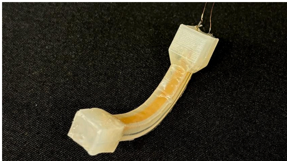
Figure 6. Fully encapsulated actuator with soldered magnetic wire leads
