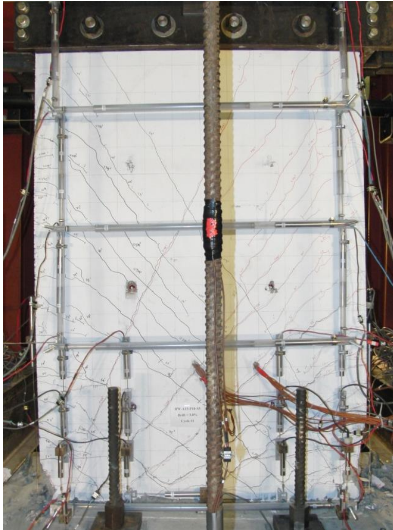
Figure A-13 Crack patterns for RW-A15-P10-S51: (a) 3.0% Drift, and (b) At end of test
