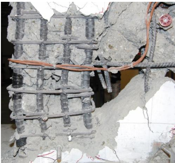
Figure 6-32 RW-A15-P10-S64: North and south wall boundaries at end of test
