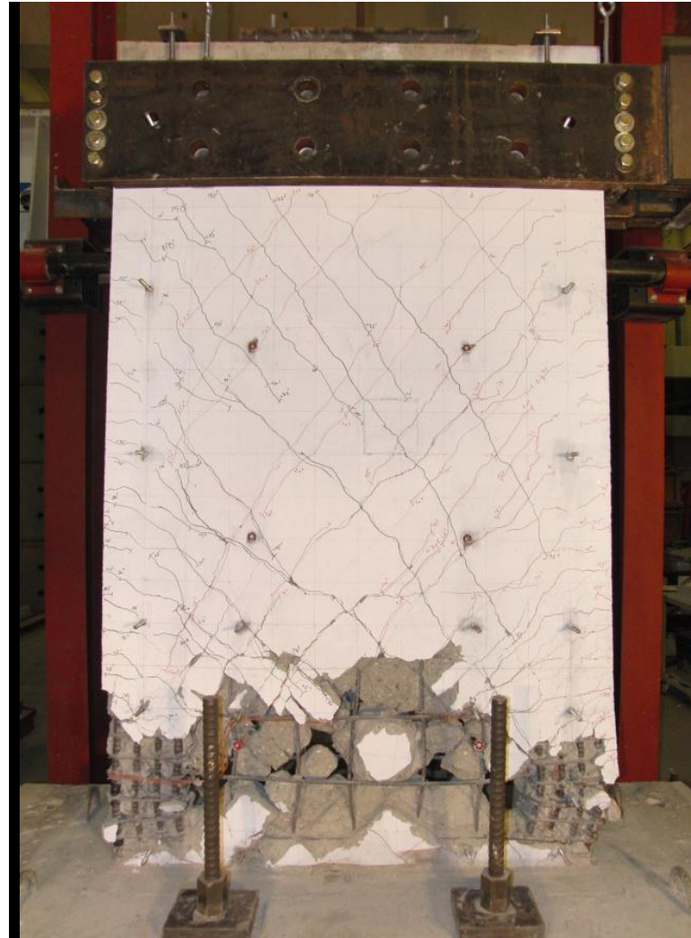
Figure A-22 Crack patterns for RW-A15-P2.5-S64: At end of test
