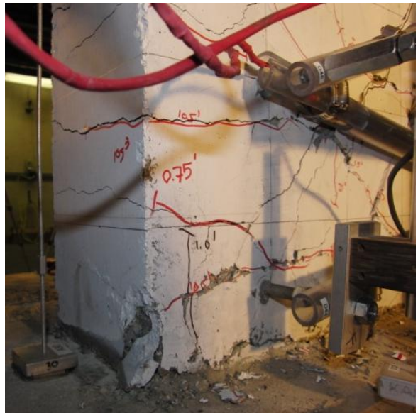
Figure 6-30 RW-A15-P10-S64: North and south wall boundaries at 1.5% drift after third cycle
