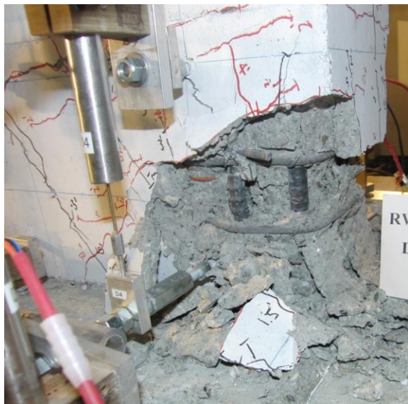
Figure 6-6 RW-A20-P10-S38: North and south wall boundaries at 3.1% drift after first cycle
