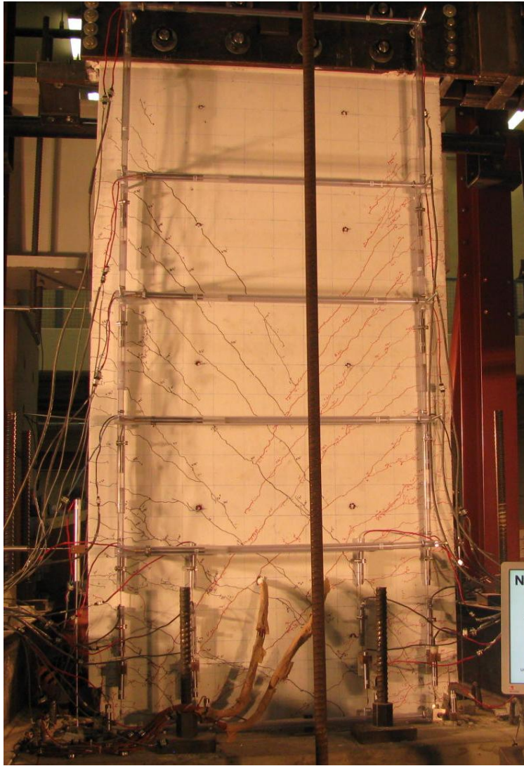
Figure A-4 Crack patterns for RW-A20-P10-S38: (a) 2.3% Drift, and (b) At end of test
