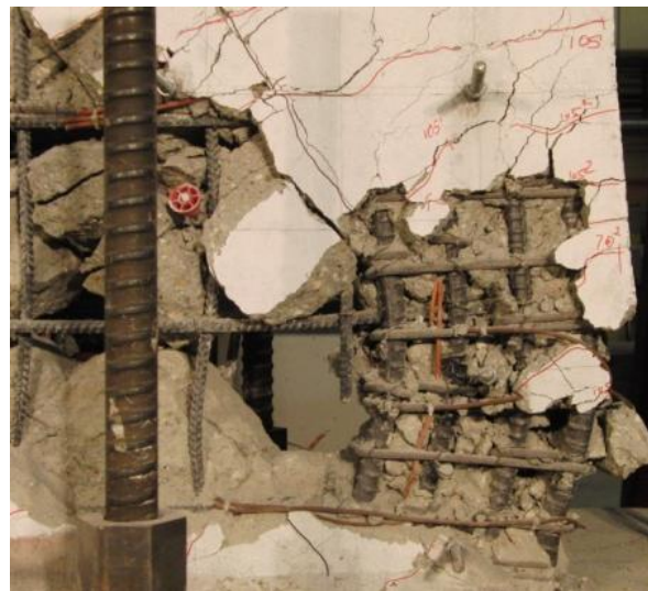
Figure 6-32 RW-A15-P10-S64: North and south wall boundaries at end of test
