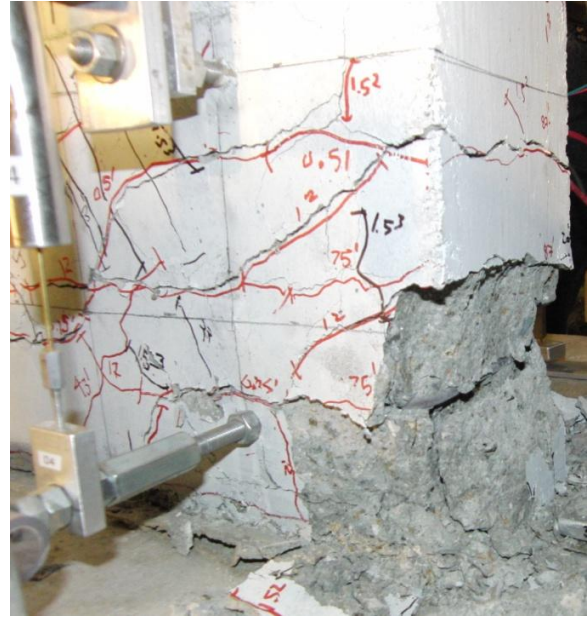
Figure 6-12 RW-A20-P10-S63: North and south wall boundaries at 3.0% drift after first cycle
