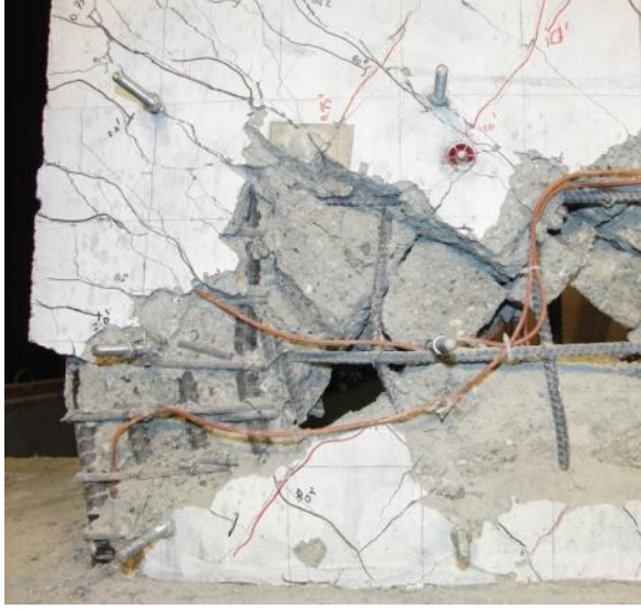
Figure 6-26 RW-A15-P10-S78: North and south wall boundaries at end of test
