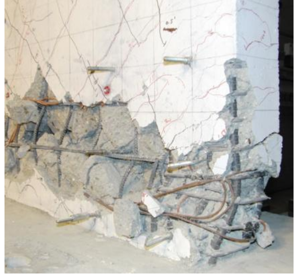
Figure 6-26 RW-A15-P10-S78: North and south wall boundaries at end of test
