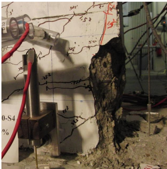
Figure 6-4 RW-A20-P10-S38: North and south wall boundaries at 1.5% drift after third cycle
