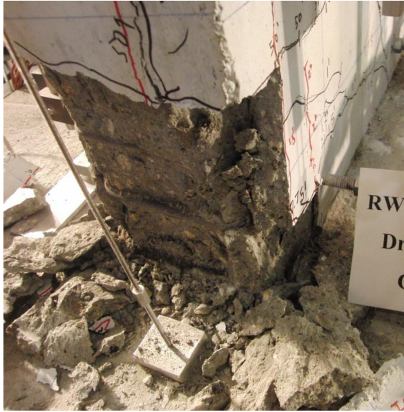
Figure 6-5 RW-A20-P10-S38: North and south wall boundaries at 2.3% drift after second cycle
