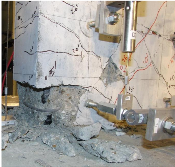
Figure 6-24 RW-A15-P10-S78: North and south wall boundaries at 2.0% drift after third cycle
