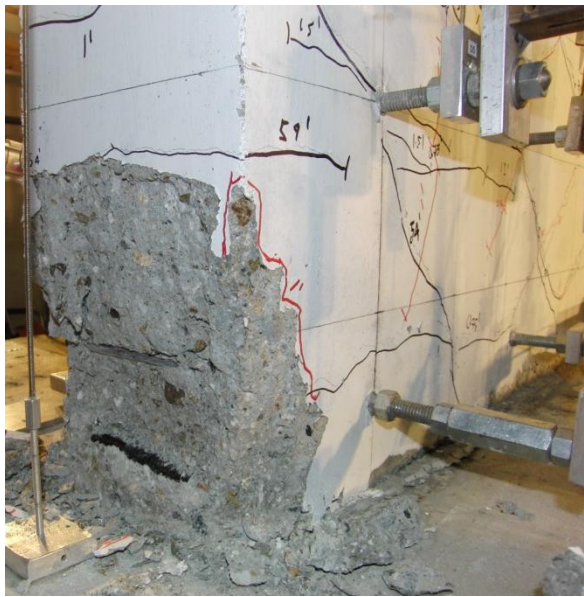
Figure 6-17 RW-A15-P10-S51: North and south wall boundaries at 1.5% drift after third cycle
