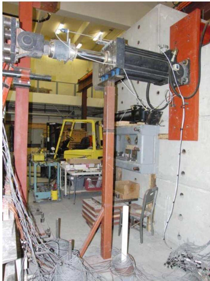
Figure 4-6 Hydraulic actuator and reaction wall
