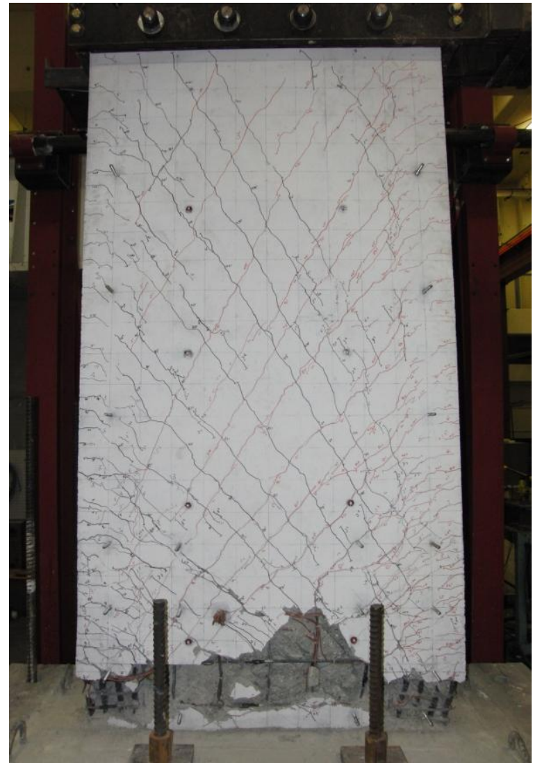
Figure A-8 Crack patterns for RW-A20-P10-S63: (a) 2.0% Drift, and (b) At end of test
