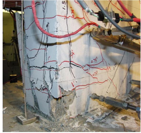
Figure 6-16 RW-A15-P10-S51: North and south wall boundaries at 1.5% drift after first cycle
