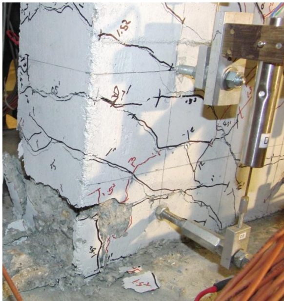
Figure 6-11 RW-A20-P10-S63: North and south wall boundaries at 2.0% drift after third cycle
