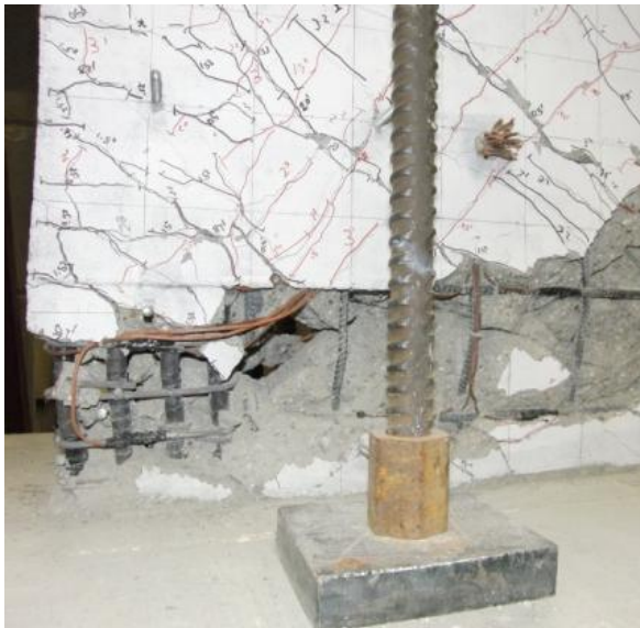
Figure 6-13 RW-A20-P10-S63: North and south wall boundaries at end of test
