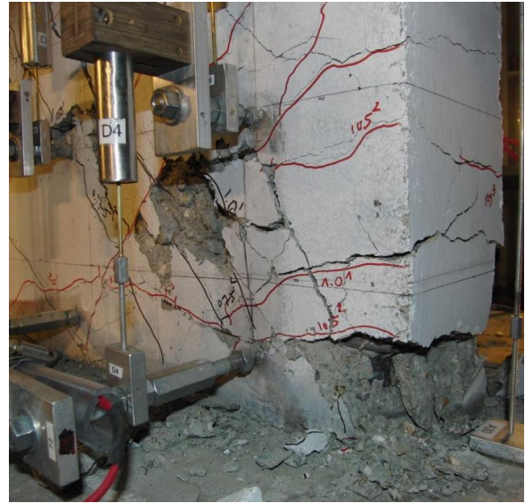
Figure 6-31 RW-A15-P10-S64: North and south wall boundaries at 2.0% drift after third cycle
