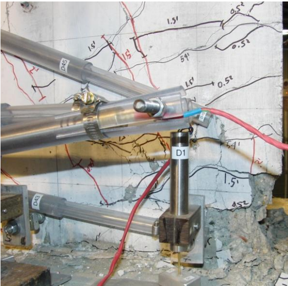
Figure 6-19 RW-A15-P10-S51: North and south wall boundaries at 3.0% drift after second cycle
