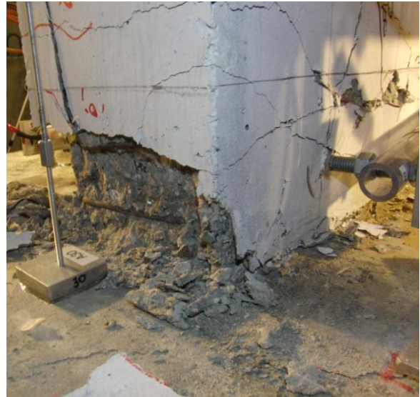
Figure 6-24 RW-A15-P10-S78: North and south wall boundaries at 2.0% drift after third cycle
