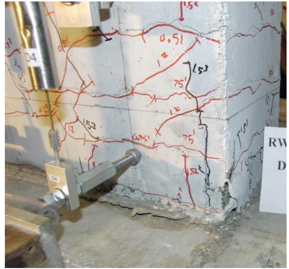
Figure 6-10 RW-A20-P10-S63: North and south wall boundaries at 1.5% drift after third cycle
