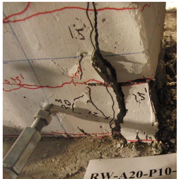
Figure 6-4 RW-A20-P10-S38: North and south wall boundaries at 1.5% drift after third cycle
