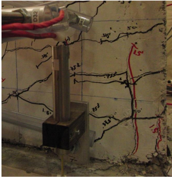
Figure 6-3 RW-A20-P10-S38: North and south wall boundaries at 1.1% drift after third cycle
