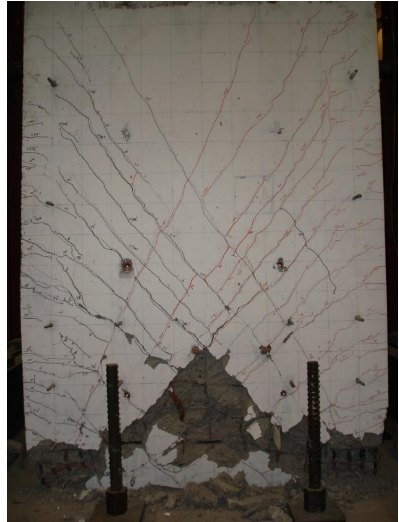
Figure A-13 Crack patterns for RW-A15-P10-S51: (a) 3.0% Drift, and (b) At end of test
