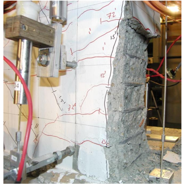
Figure 6-17 RW-A15-P10-S51: North and south wall boundaries at 1.5% drift after third cycle
