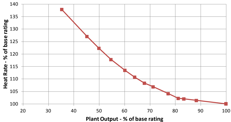
Figure 94 - Part-Load Performance of a GE STAG 209E Combined Cycle Generator [38] (two turbines)
