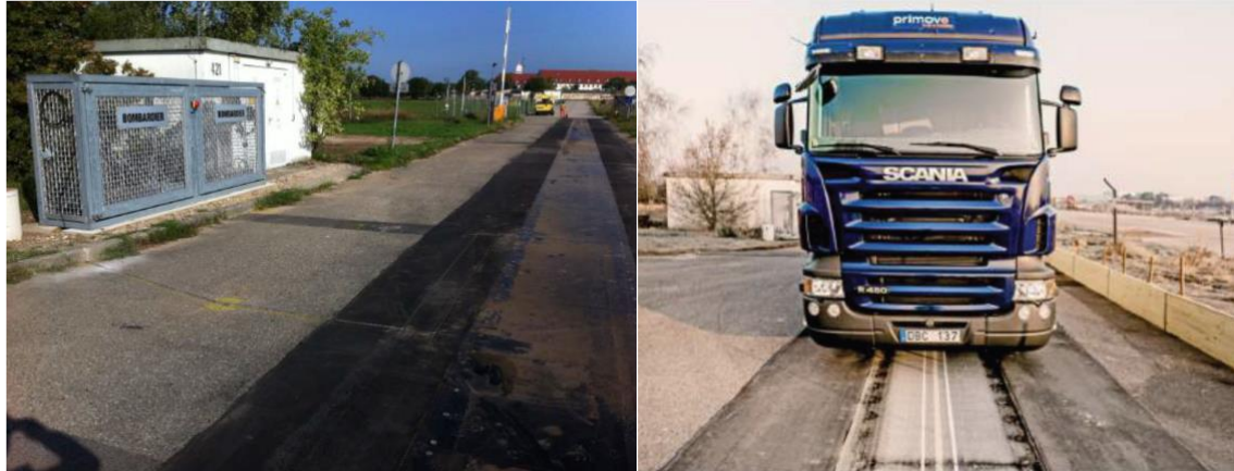
Figure 10. Electrified test track with PRIMOVE and Scania Truck [Source: Sweden Viktoria ICT]
