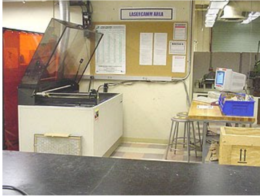
Figure 3.4: LaserCamm used to fabricate the substrates
