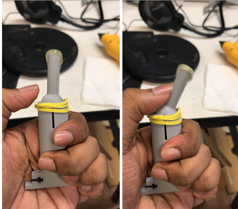
Figure 4.1: New Foot design with 30Deg of compliance
