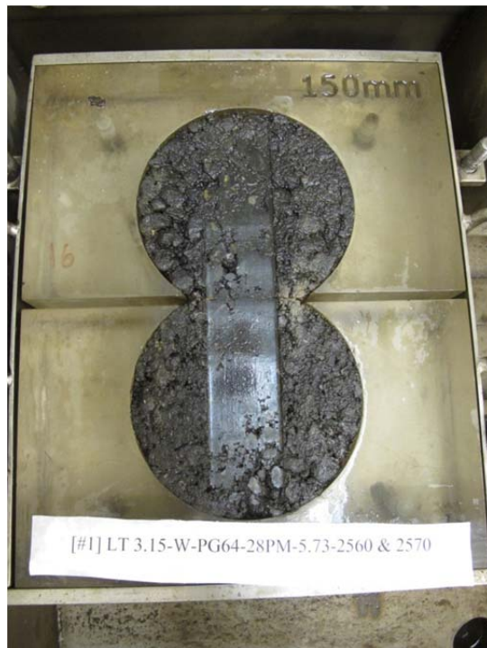
Figure C.4: HWTT result for PG 64-28PM 15% RAP, 1.2% lime (set #2, lt.) after 22,950 passes.
