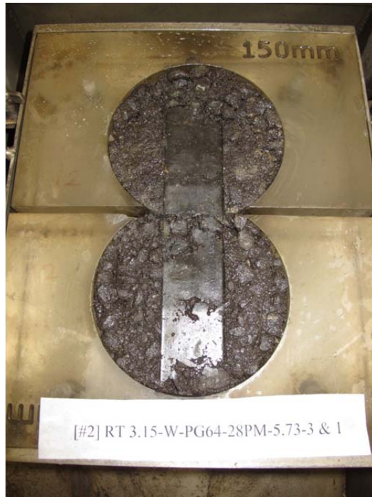
Figure C.3: HWTT result for PG 64-28PM 15% RAP, 1.2% lime (set #2, rt.) after 22,950 passes.
