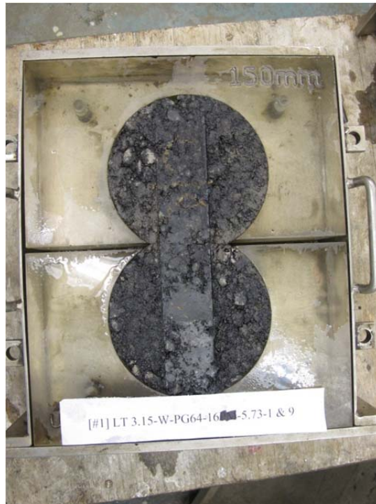
Figure C.7: HWTT result for PG 64-16 25% RAP, 1.2% lime (set #2, rt.) after 40,000 passes.
