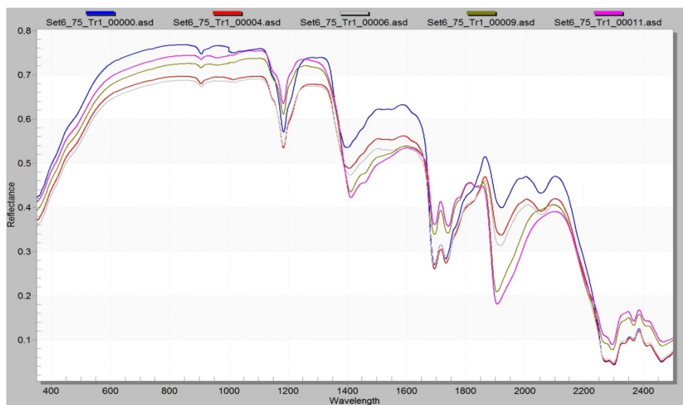
Fig. 26: Reflectance spectra for Trial 1 with main absorption features in the NIR
