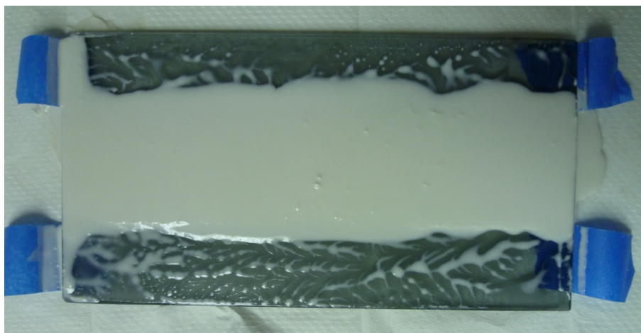
Fig. 11: Aspect of the film after removal of the Plexiglas stripes from the glass plate
