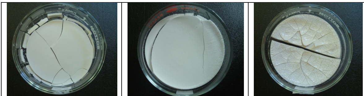
Fig.13: Samples showing no separation (++), minor separation (+), and clearly visible separation (-). Separation is evident where particulate has sunk to the bottom of the dish, leaving the transparent, glassy surface of the silica at the top, and resulting in crizzling and sometimes peeling of the top layer. The center sample shows partial separation at the right side of the dish, where minor crizzling has occurred in a localized area.
