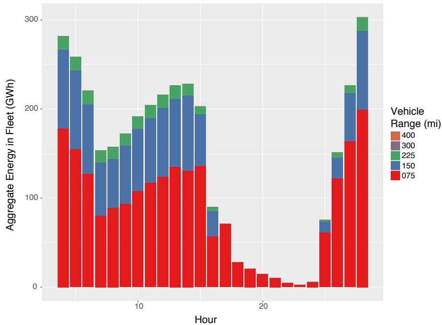
Figure 7.7: Aggregate energy stored in national fleet batteries by vehicle range by hour of day.
