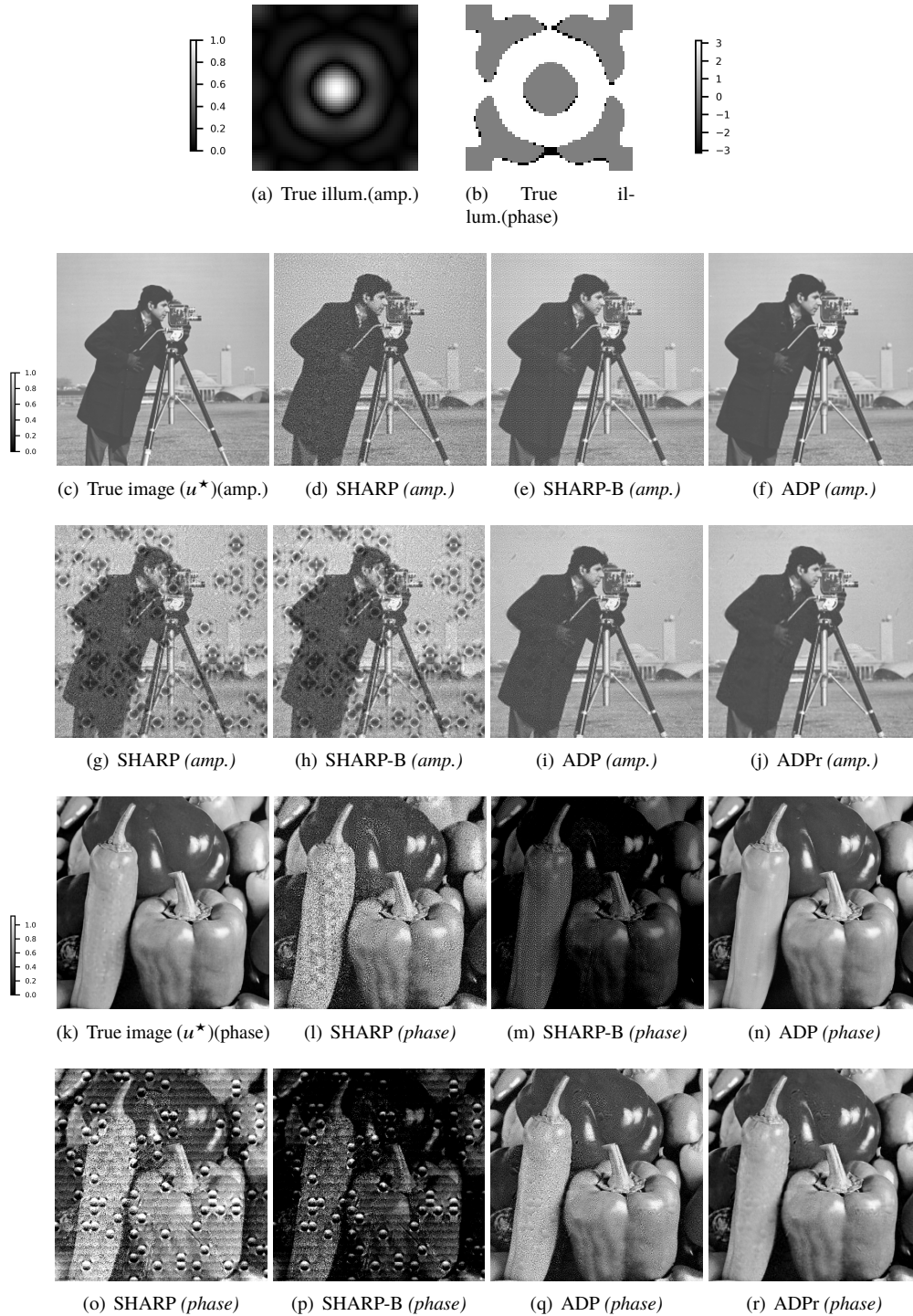
Fig. 2. Simulation experiment. First row: (a)-(b) Amplitude and phase for true illumination (illum., 64 \times 64 pixels), with Full Width at Half Max (FWHM) = 7 pixels. Second row: Amplitude of true image (c) with 496 \times 496 pixels, and amplitude of recovered images with data contaminated by only parasitic noise, using SHARP (d), SHARP-B (e) and ADP (f). Third row: Amplitude of recovered images with data contaminated as in Eq. (32) and also by additional outliers, using SHARP (g), SHARP-B (h), ADP (i), and ADPr (j). The fourth, and fifth rows show the corresponding phase parts of the images in the second and third rows.
