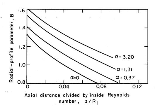
Fig. 7. Radial parameter of the axial velocity as a function of jet length and density-viscosity product ratio.
