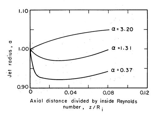
Fig. 8. Jet radius as a function of jet length and density-viscosity product ratio.
