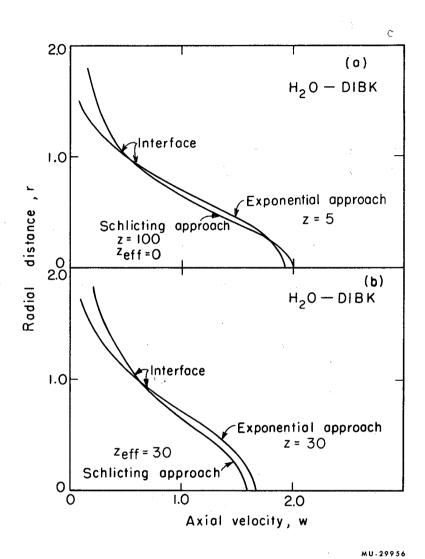
Fig. 12. Comparison of exponential and Schlicting-type velocity profiles; water into di-isobutyl ketone; (a) z = 5, z(eff) = 0, (b) z = 30.
