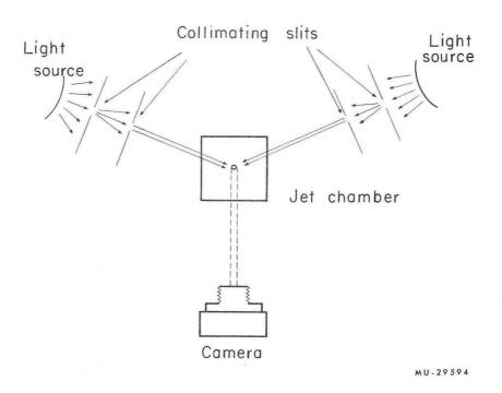
Fig. 15. Illumination diagram with camera position.
