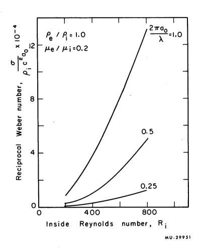
Fig. 4. Relation between dimensionless parameters defining oscillating-jet behavior. Density ratio, 1.0; viscosity ratio, 0.2.
