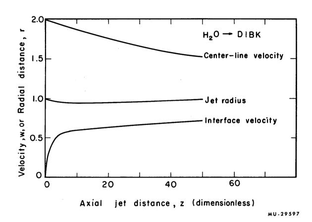
Fig. 9. Center-line and interface velocity and jet radius as function of jet length ( $\alpha$  = 0.74).
