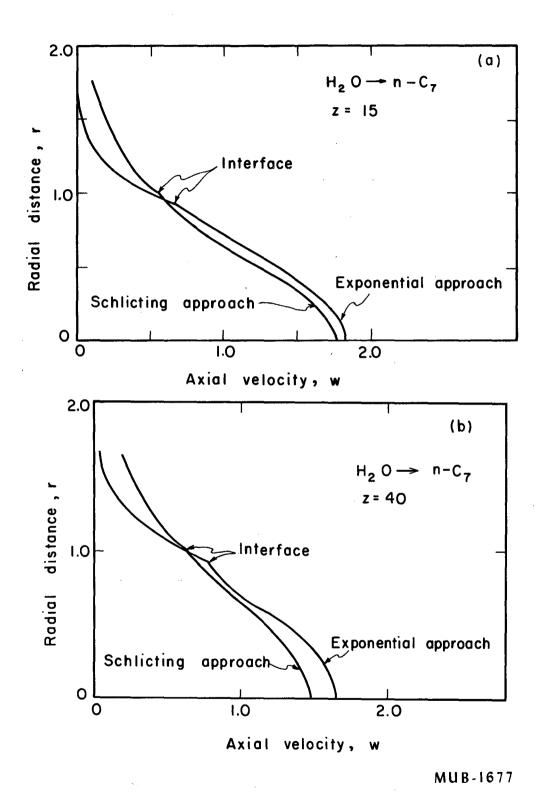
Fig. 11. Comparison of exponential and Schlicting-type velocity profiles; water into normal heptane; (a) z = 15, (b) z = 40.
