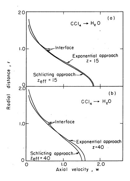
Fig. 10. Comparison of exponential and Schlicting-type velocity profiles; carbon tetrachloride into water; (a) z = 15, (b) z = 40.
