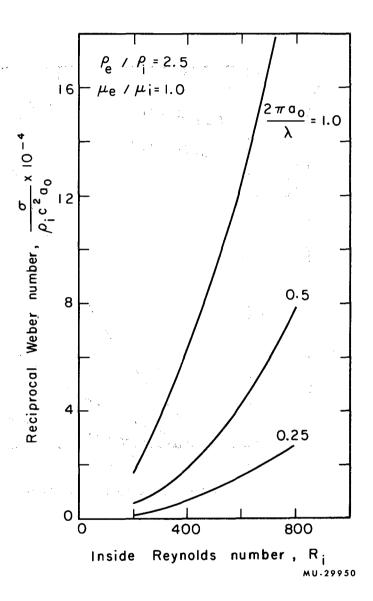
Fig. 3. Relation between dimensionless parameters defining oscillating-jet behavior. Density ratio, 2.5; viscosity ratio, 1.0.
