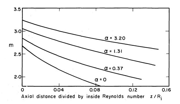
Fig. 6. Center-line velocity parameter as a function of jet length and density-viscosity product ratio.
