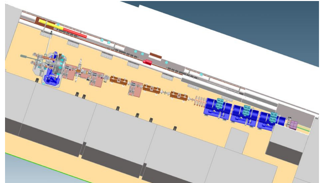
Figure 1: APEX Facility Layout. The electron gun is on the top-left part of the figure while the dark cylinders in the bottom-left are the three undulator cryostats. The total length of the shielded area is about 15 m.
