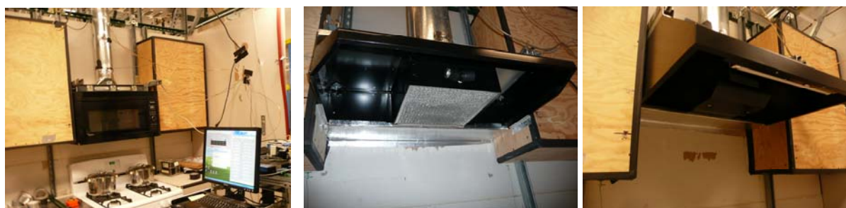
Figure 1. Exhaust hoods A, B, C shown from left to right; test area shown in left panel.
