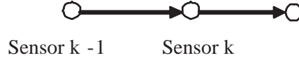
Figure 2.1: Portion of a routing path where each sensor has only one upper stream sensor.
