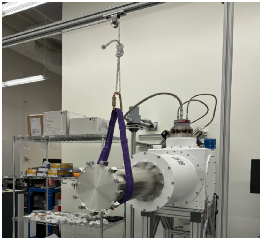
Figure C.15: Vacuum nipple attached to Snoopy and resting in sling of pulley system.
