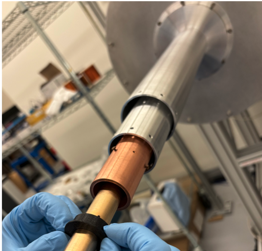
Figure C.12: Sliding the alignment piece out of the cold fingers after inserting Vespel screws. 4 K and 40 K shields are already attached.
