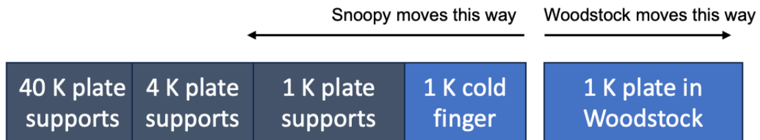
Figure B.4: Simplified model for 1 K contraction calculations. Snoopy components are on the left and Woodstock components are on the right.
