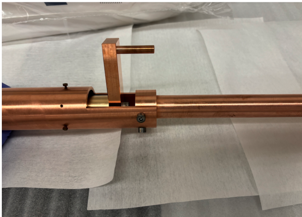
Figure C.4: V-bar attached to the 20 mK cold finger. Note that in this photo, the Vespel screws are already inserted; this was done before the assembly ring method was adopted.
