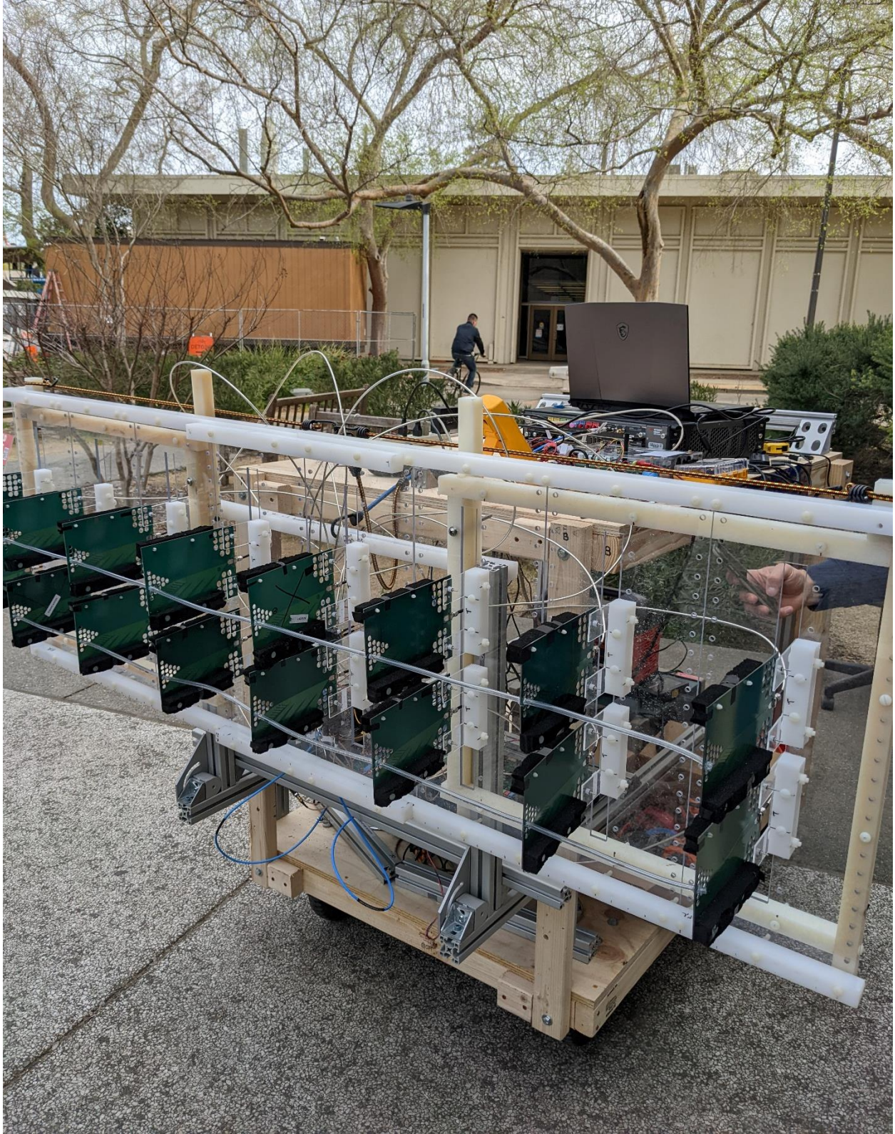
Fig. 67. Cart “skyshot” configuration – used to take calibration and coupling waveforms between each antenna pair.
