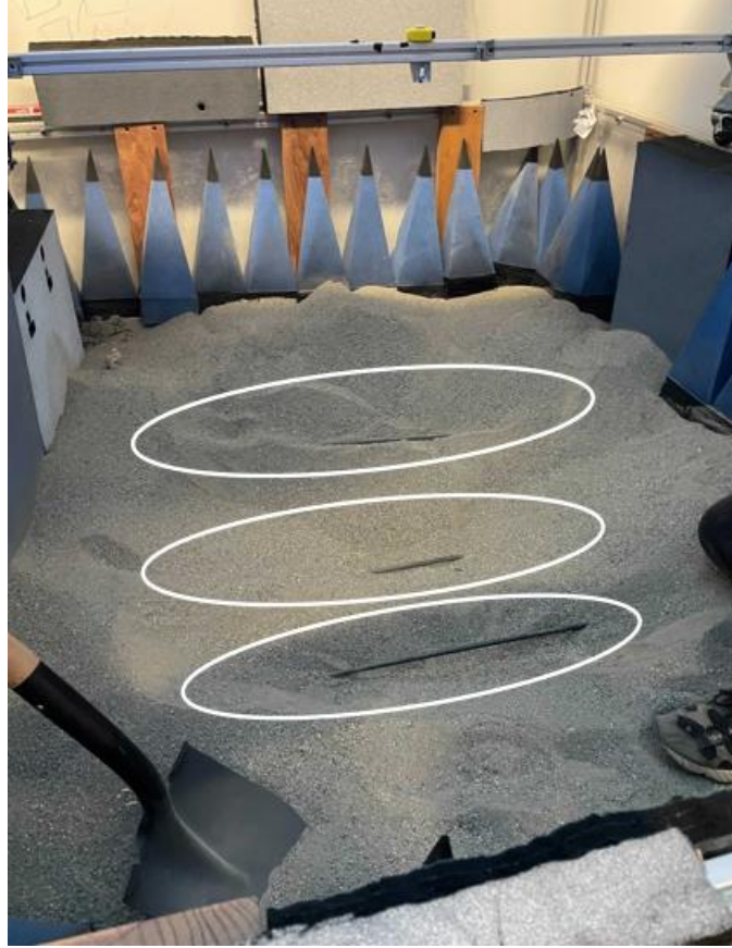
Fig. 68: Sandbox with half-buried rebar targets. Targets are fully buried later to depths of Fig. 69.
