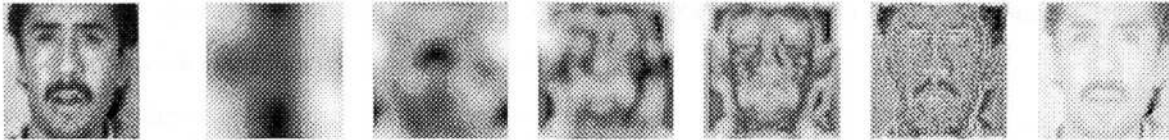
Figure 2: Original image and Gabor jets at six scales. Each pixel's intensity in the processed images represents the log of the sum of the magnitudes of the filter responses in each of the eight directions.
