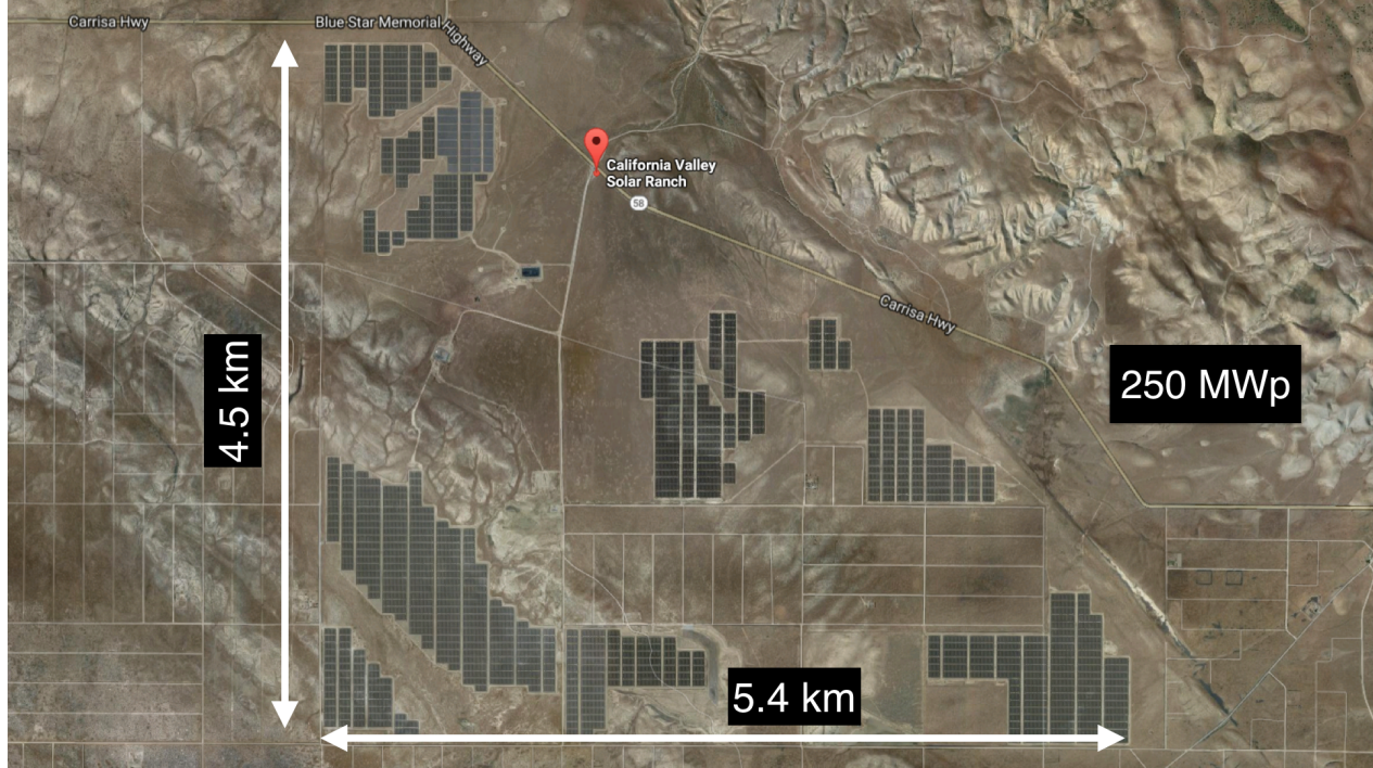
Figure 1.1: An annotated satellite view of the 250 MW p California Valley Solar Ranch (CVSR). The sites covers approximately 17 km 2 , although the area covered by solar panels is less than half of that size ( \approx 8 km 2 ).
