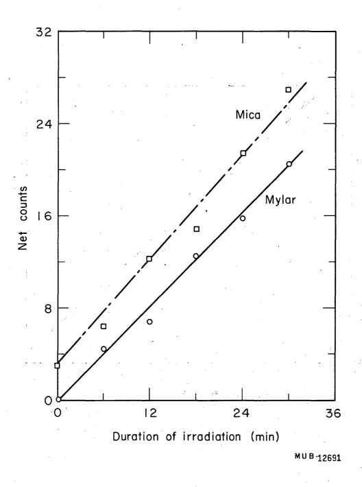
Fig. 3. Net counts for mica and Mylar as functions of irradiation time under natural uranium 1.8 cm from a PuBe source giving  $8.6\times10^7$  n/sec.
