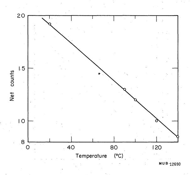
Fig. 4. Counts as a function of annealing temperature; Mylar, irradiated and annealed 30 min at various temperatures.
