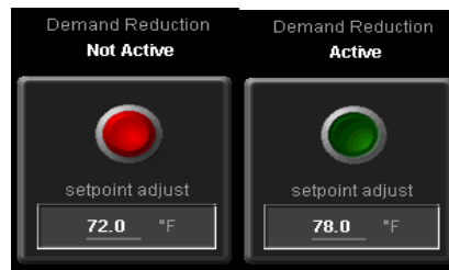
Figure 1. GEMnet demand response control interface.
