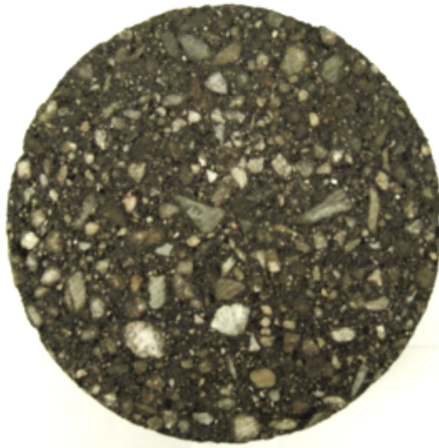
Figure 3.2 Plan view of asphalt concrete cylinder cast with innovative asphalt materials
