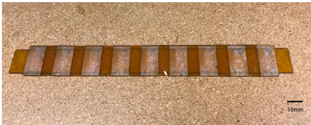
Figure 5.2 A long SLL prototype used for wind tunnel testing
