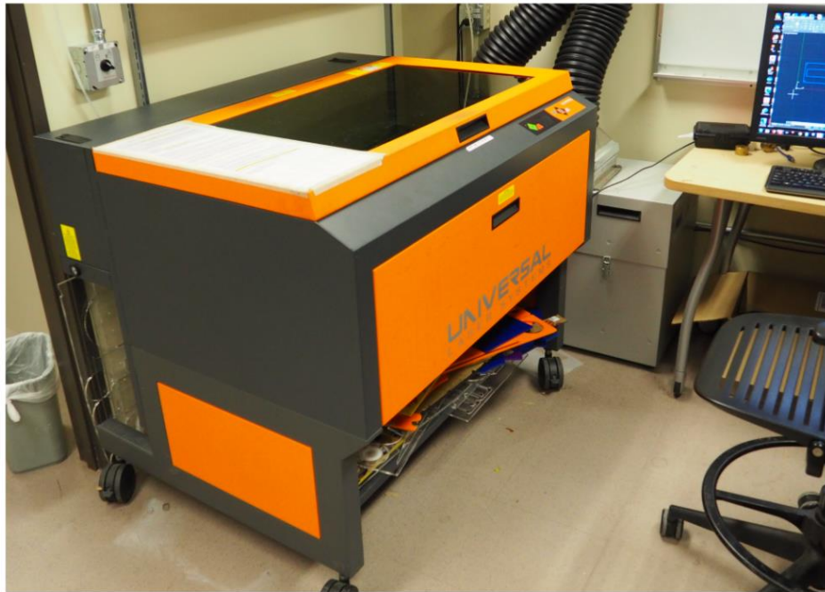
Figure 3.2 The UNIVERSAL® laser system for SLL fabrication from Prof. Tolley's lab.
