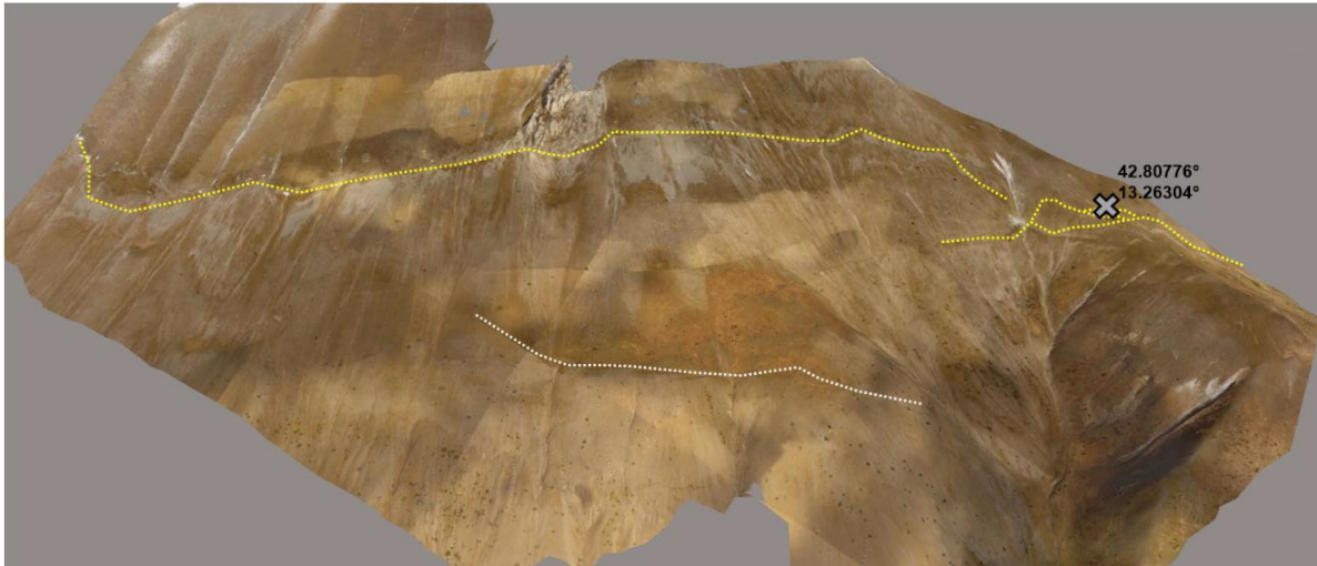
Figure 4. UAS/TLS-based orthomosaic model of the SW face of the Mt. Vettore Massif after the 30 October earthquake with 3D digital terrain model from merged SfM and LiDAR data. Approximate main fault trace(s) indicated in yellow, a second 1 km long visible trace of the “Western Trace” shown in white. Looking from the west. The left of the image is to the north. The slope moves from top to bottom of the image.
