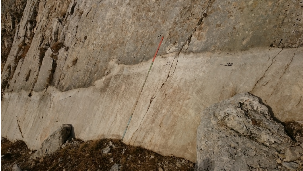
Figure 6. Example of fault slip measurements showing multi-epoch offsets from August 2016 (upper white band, 16 cm) and October 2016 (130 cm) events. Lat = 42.81724, Long = 13.25449.
