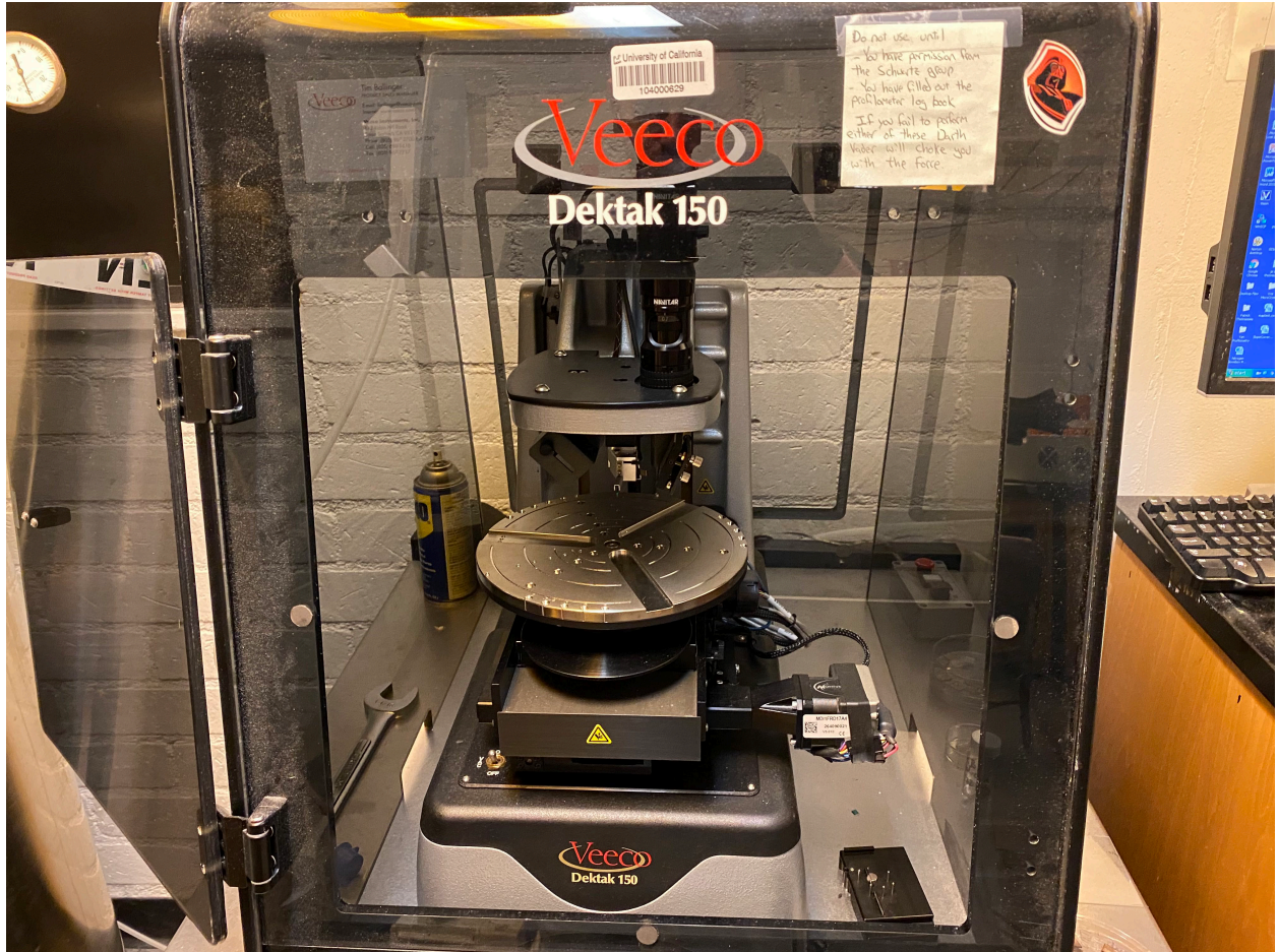
Figure D.1: View of our Veeco Dektak 150 Surface Profilometer from the front.
