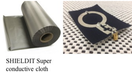
Figure 3.15: The electro-textile coil element using conductive cloth SHIELDIT Super. The coil element pattern is laser cut and attached to the cotton cloth using adhesive material. The electronic components are soldered onto the surface with controlled temperature.
