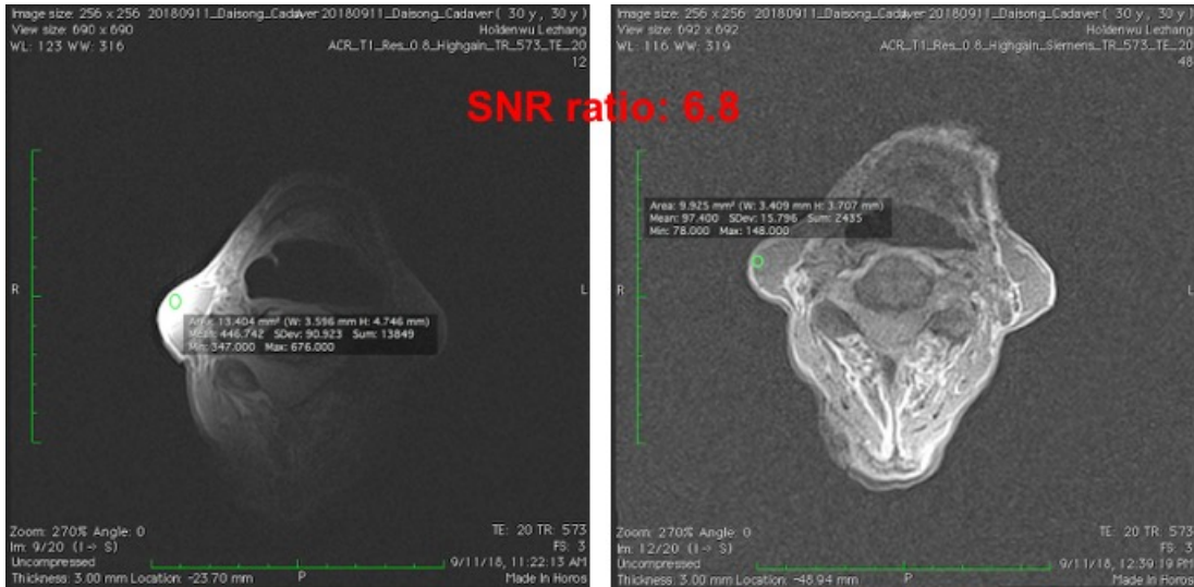
T1 weighted spin echo Siemens 4-channel Flex coil, SNR=49.3
