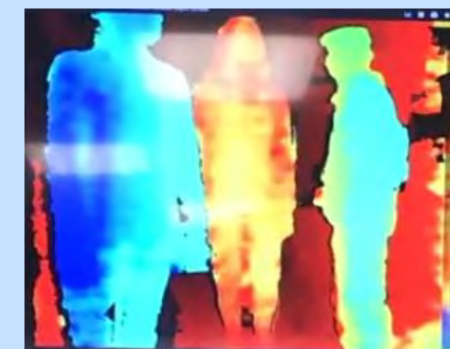
Figure 3: Depth algorithm color mapping where red represents farther distances and blue, closer
