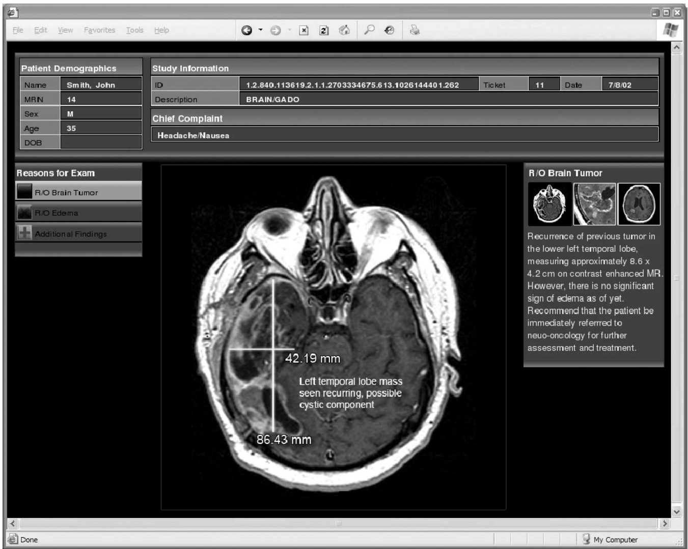
Fig. 6. Web-based results view display created for the openSourcePACS primary care/specialist communication loop application (patient information is fictitious). When a radiologist completes the preliminary review, the system generates a website that pulls together the DICOM presentation states (PS) and comments in the associated DICOM structured reporting object. Patient demographics and study information are presented at the top of the interface. The reasons for exam and the radiologist's answers are given in the left-side panel with icons (in this case, a brain tumor was found, thus indicated by a check mark; edema was not found, indicated by "X"; and additional findings are given). Selecting a reason for exam on the left, calls up the image slices chosen by the radiologist. The DICOM PS is shown in the middle of the display. Additionally, related image slices selected by the radiologist can be seen by choosing from the thumbnail views on the right.
