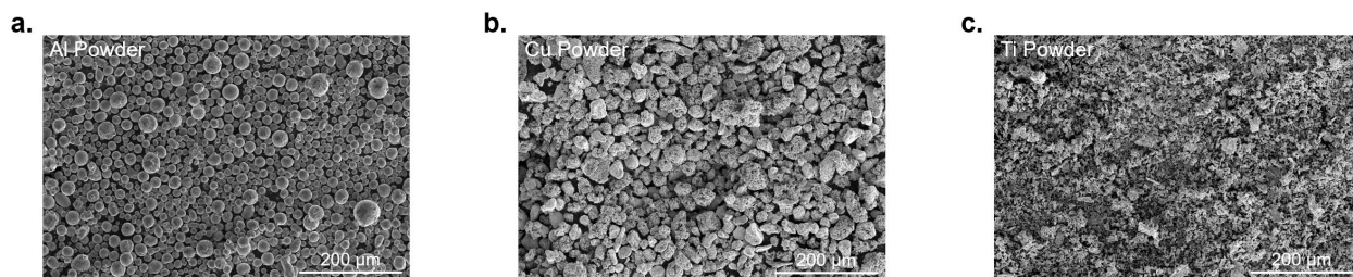
Supplementary Figure 17. Particle morphology evaluated by SEM for a) Al, b) Cu, and c) Ti powders.
