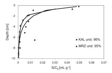
**Fig. 3.** Observed and simulated retention profiles for MWCNT in an undisturbed silty loam soil from the test site in Merzenhausen (MRZ) compared with the previously shown RP for the undisturbed loamy sand soil from the test site in Kaldenkirchen-Hülst (KAL). The water-saturation was around 96%. For detailed experimental conditions see Table 2. The dots are the experimental data and the lines represent the model fits.
