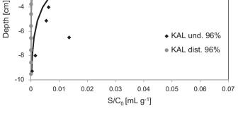
**Fig. 2.** Observed and simulated retention profiles for MWCNT in a disturbed (dist.) soil column from the test site in Kaldenkirchen-Hülst (KAL) compared with the previously shown RP for the undisturbed soil column from the same test site. The water-saturation was around 96%. For detailed experimental conditions see Table 2. The dots are the experimental data and the lines represent the model fits.
