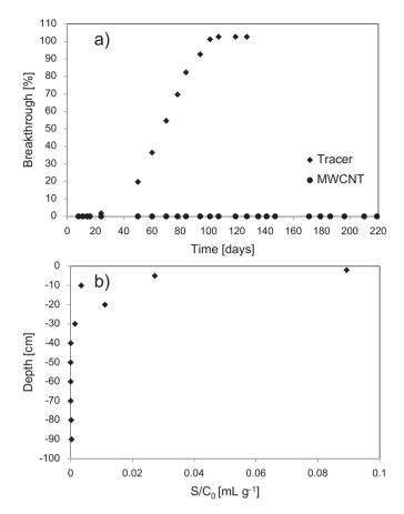
**Fig. 4.** Cumulative breakthrough of tracer (Br<sup>-</sup>) and radiolabeled MWCNT (a) as well as an averaged retention profile (b) 220 days after application of MWCNT to a lysimeter. The lysimeter was filled with an undisturbed loamy sand soil from the test site in Kaldenkirchen-Hülst.
