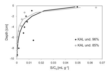
**Fig. 1.** Observed and simulated retention profiles for MWCNT in undisturbed (und.) loamy sand soil cores from the test site in Kaldenkirchen-Hülst (KAL) at two water-saturation levels (85 and 96%). For detailed experimental conditions see Table 2. The dots are the experimental data and the lines represent the model fits.
