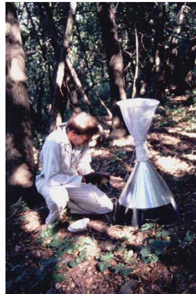
Duplex cone trap baited with dry ice, being tested by UC Berkeley entomologists to capture adult western treehole mosquitoes seeking blood meals, Spring 1991
