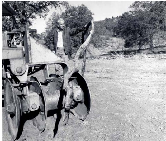
Al Murphy with range brush disk used in vegetative conversion of chaparral, James III Pasture, October 1971
