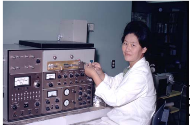
Lee U. Oh with gas chromatograph used in analysis of volatile fatty acids in rumen samples, June 1972
