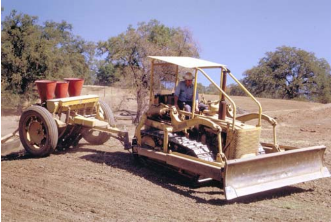
Range drill and bulldozer used in seeding for improved pasture, October 1972
